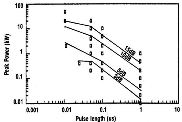
Figure 5. First pulse damage profile (power versus pulse length).
