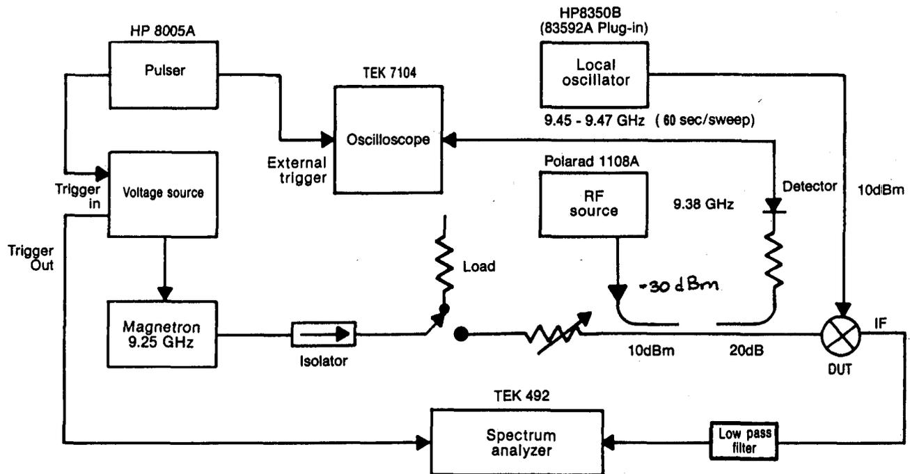
Figure 1. Block diagram of mixer diode damage setup.
