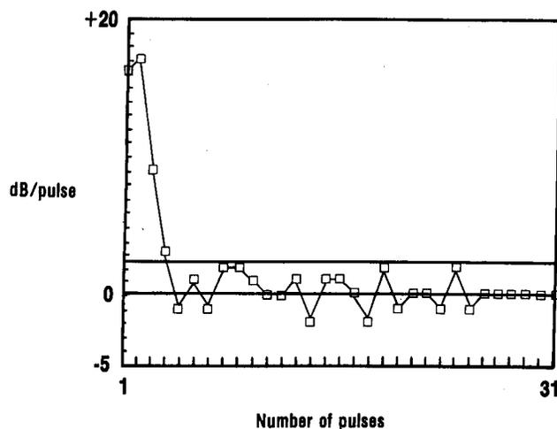
Figure 4. Damage differential versus the number of pulses for 1 us, 1 kW, 9.25 GHz pulse response.
