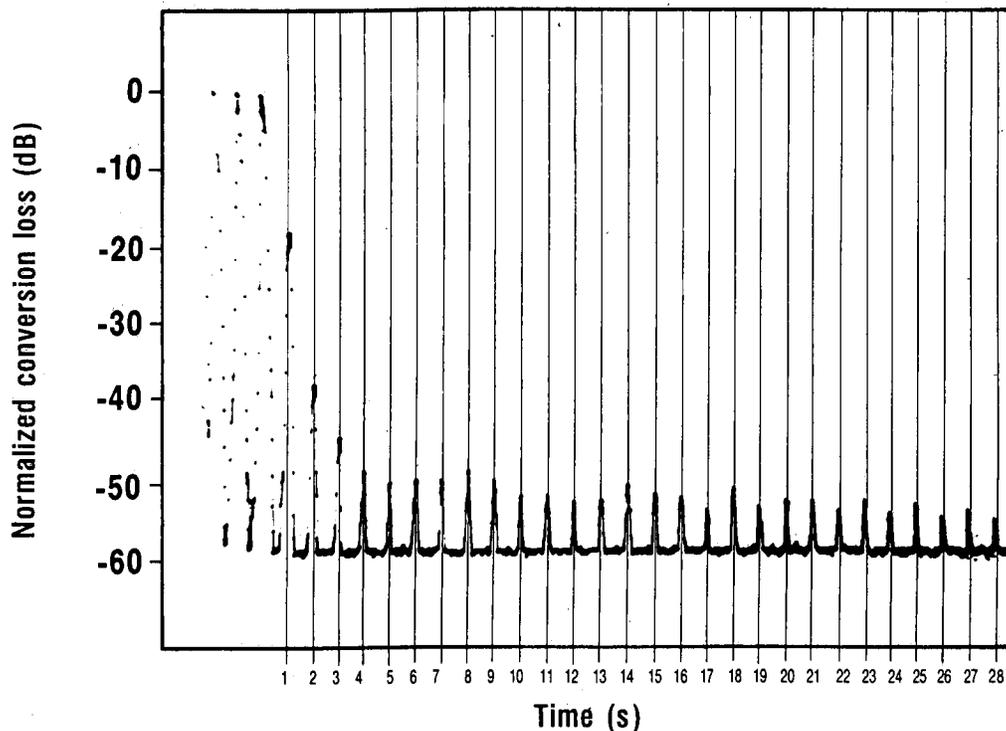
Figure 2. Spectrum analyzer display of mixer response to 1 microsecond, 1 kW, 9.25 GHz pulses.
