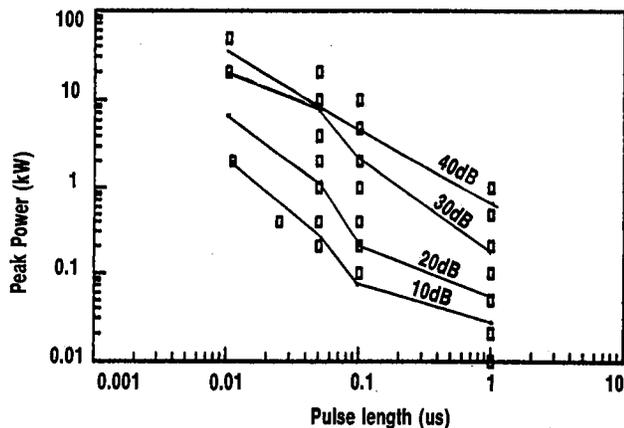
**Figure 6. Final damage profile (power versus pulse length).**
