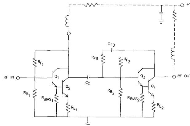
Figure 2. Circuit schematic for the 20dB gain/20dBm power output, hybrid, cascaded amplifier.
