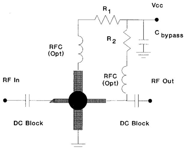
**Figure 3. Amplifier lead connections and bias configuration.**
