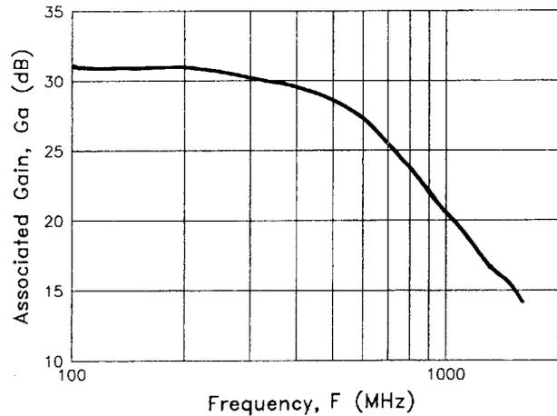
Figure 5. Hybrid amplifier associated gain versus frequency.
