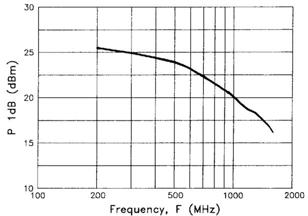
Figure 6. Hybrid amplifier 1dB power compression point versus frequency.
