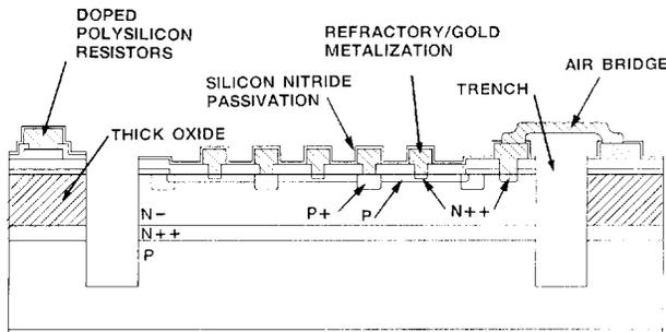
Figure 8. Cross section of isolated collector structure.
