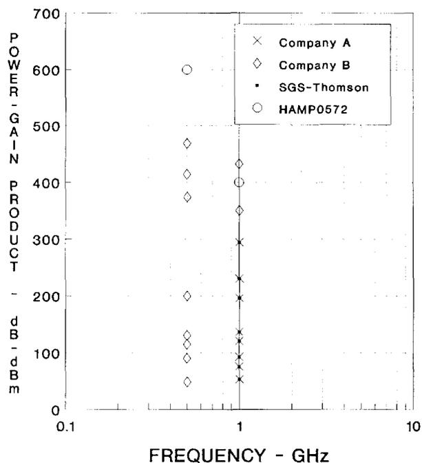
Figure 1. Available silicon MMIC amplifiers' power-gain products versus frequency.
