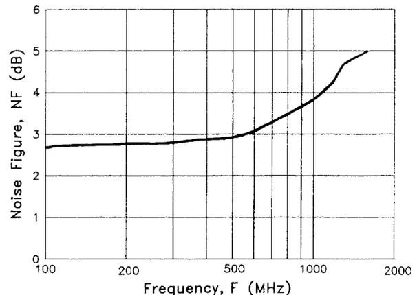
Figure 7. Hybrid amplifier noise figure versus frequency.
