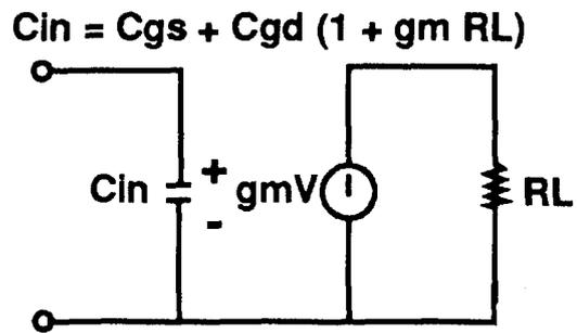
Figure 3. Further simplified model with equivalent input capacitance.
