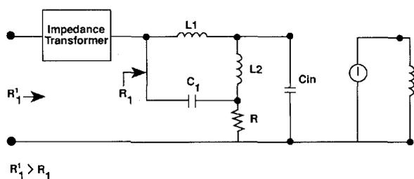
Figure 6. Matching approach for large periphery FET.
