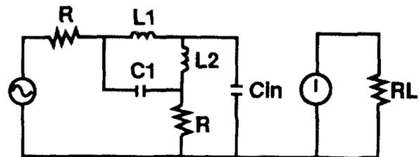
Figure 4. All-pass filter matching network.
