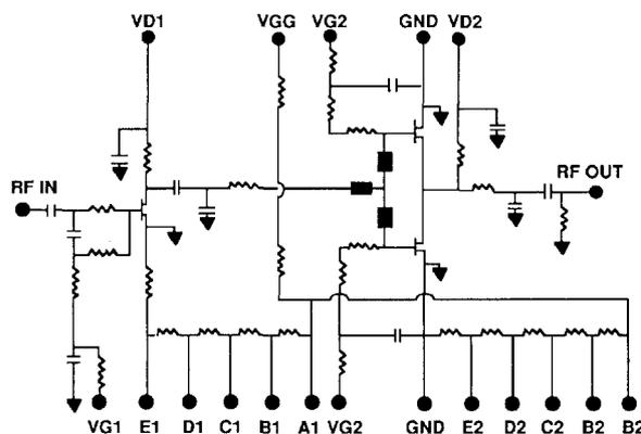
Figure 7. Simplified schematic of the Amplifier Chip.
