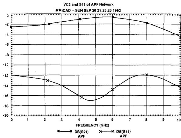
Figure 5. Gain compensation and impedance match of 1.2mm FET using all-pass network.
