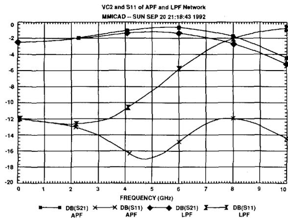
Figure 8. Comparison of all-pass network and low-pass network gain compensation and impedance match for 1.2mm FET.
