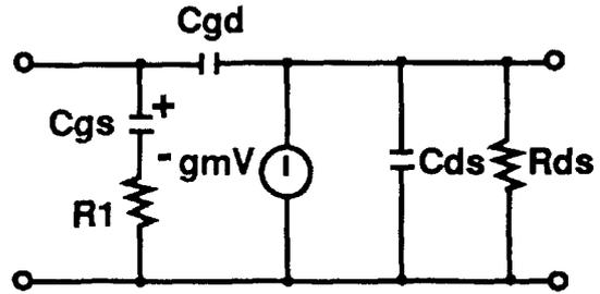
Figure 2. Simplified MESFET Linear Model.
