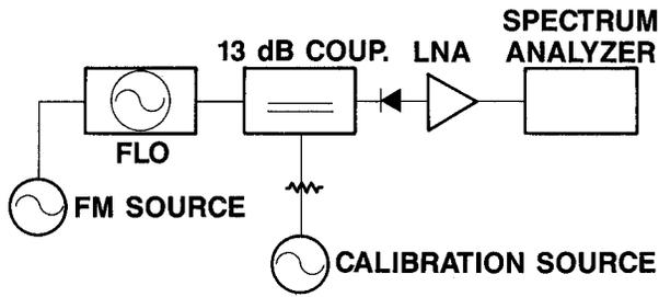
Figure 5. The test setup used for measuring residual AM.
