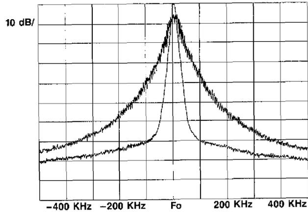
Figure 4. Oscillator noise spectral density under open and closed loop conditions. The center frequency was 9.6 GHz, residual bandwidth 10 KHz and the viewing bandwidth 100 Hz.
