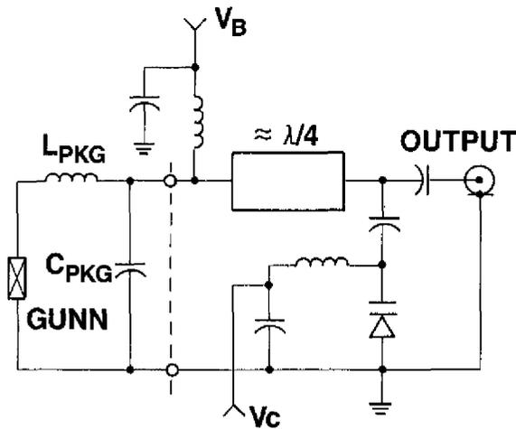
Figure 2. Schematic of the low Q Gunn oscillator with varactor tuning.
