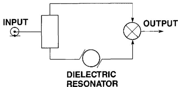
Figure 3. Block diagram of the balanced mixer frequency discriminator.
