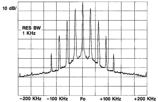
Figure 6. The measured FM sidebands of the frequency locked loop.
