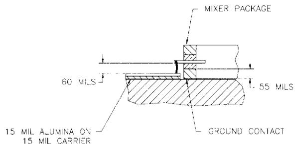
Figure 2. Typical mixer package mounted to ground plane.
