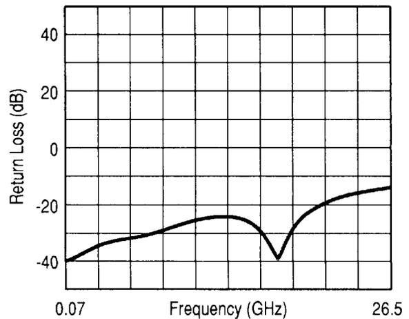
Figure 9d. Gated (calculated) return loss of a single package transition.
