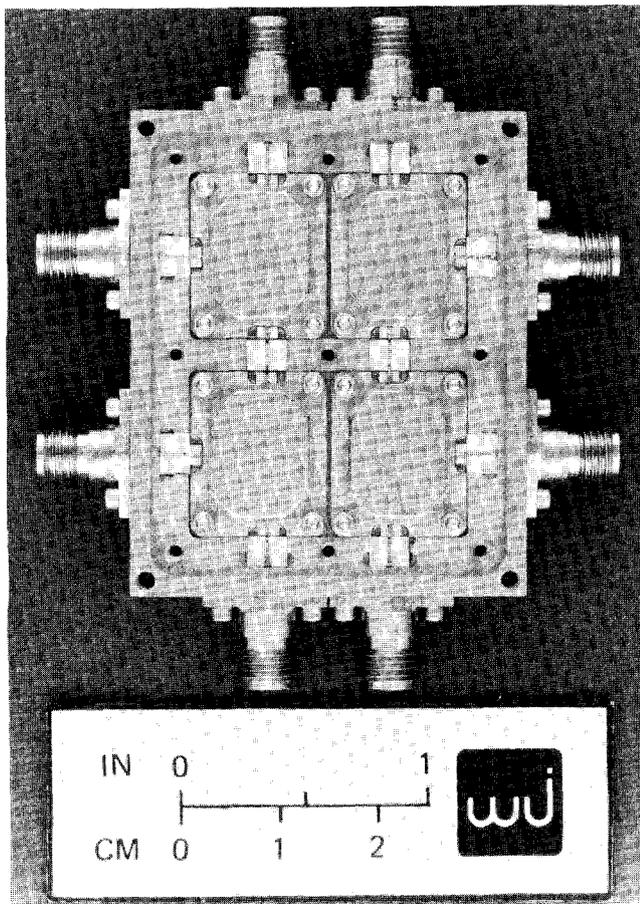
**Figure 10. Photograph of multiple package test circuit. Two channels are provided so that isolation measurements can be performed.**
