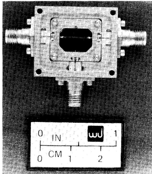
Figure 8. Photograph of the new hermetic mixer package mounted in a microstrip test fixture. Lid is removed and 50 ohm line installed for test purposes.
