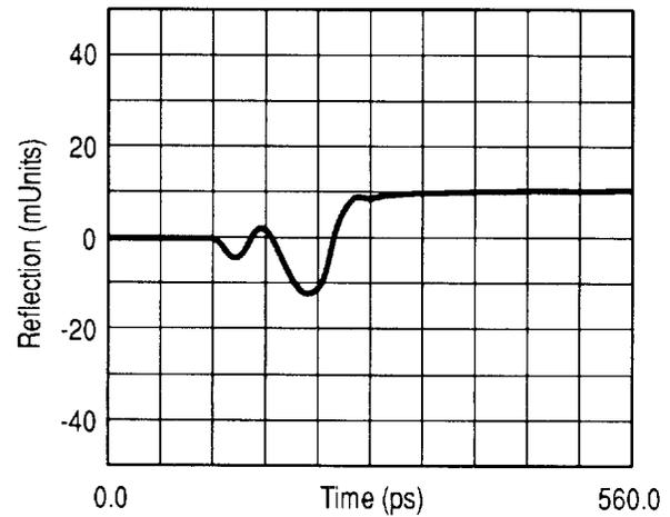
Figure 9c. Gated (calculated) time domain reflection of a single package transition.
