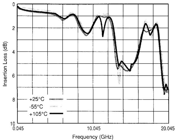
**Figure 13. Insertion loss obtained with a conventional package, showing a practical limit of about 12 GHz.**
