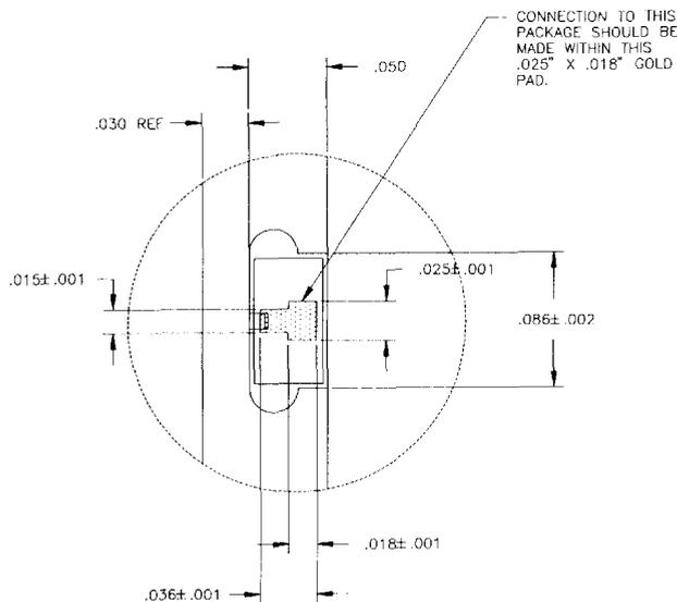
Figure 7. Details of the microstrip interface.
