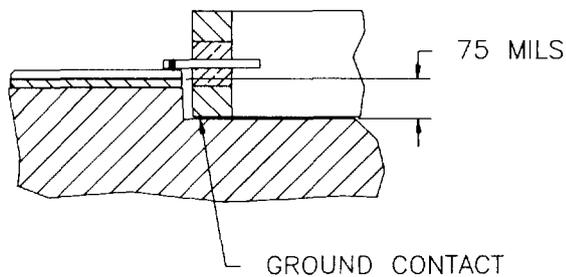
Figure 3. Typical mixer package mounted in cavity.
