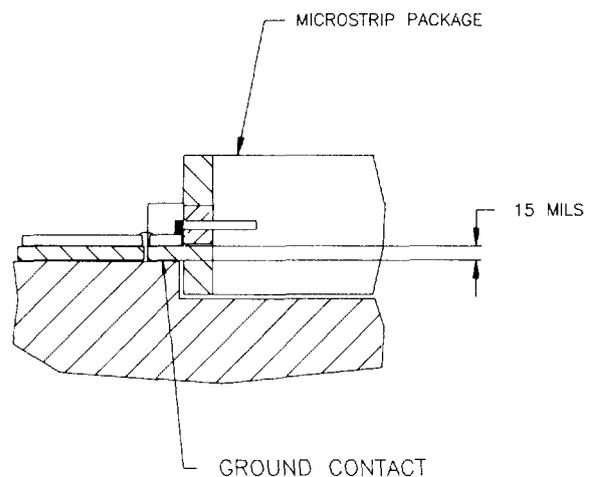
Figure 5. Side view of a microstrip package mounted in subsystem.
