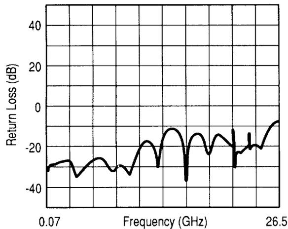
Figure 9b. Return Loss (reflection) over frequency of the package and test fixture.
