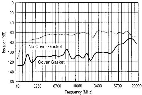
**Figure 12. Measured isolation between channels, with and without package lids, using the test fixture of Figure 10.**
