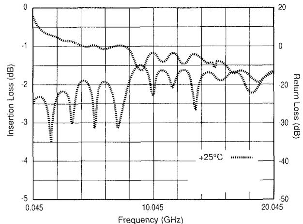
**Figure 11. Insertion and return loss for one channel of the test fixture shown in Figure 10.**
