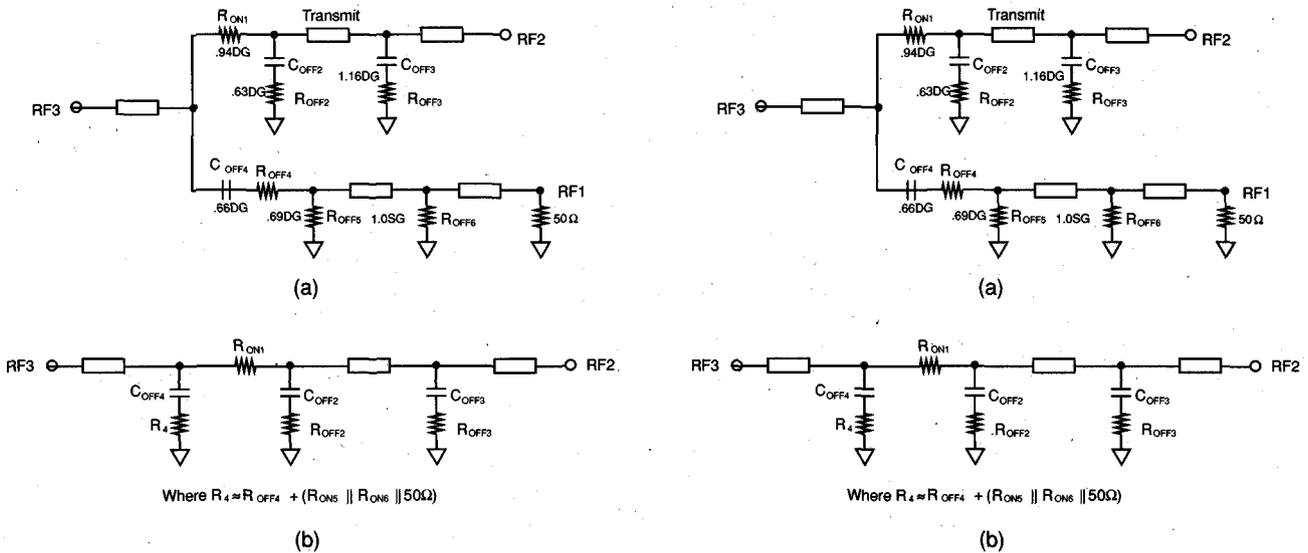
**Figure 2 (a) Complete equivalent circuit of the switch in Transmit mode, (b) simplified equivalent circuit.**
