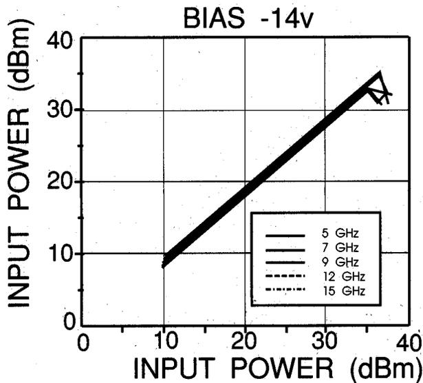
Figure 6. Power transfer curves for the T/R switch in Transmit mode; output versus input power is shown.
