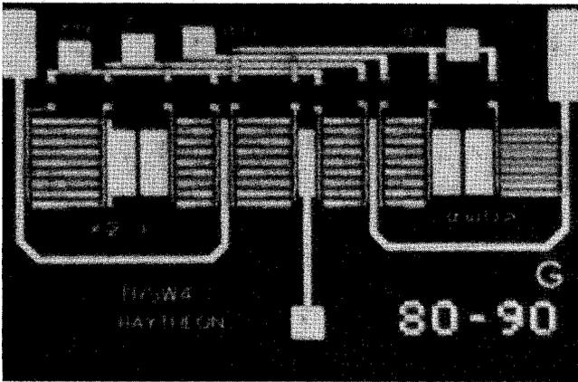
Figure 4. Photograph of the 2-18 GHz high power switch.
