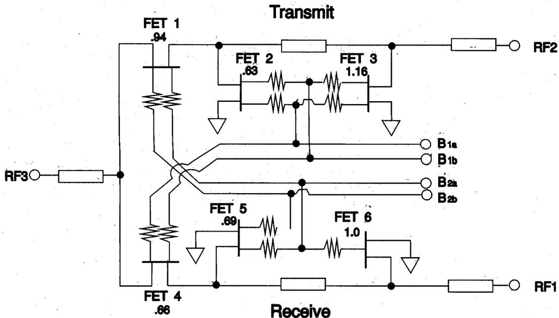
Figure 1. Schematic of the 2-18 GHz high power T/R switch.
