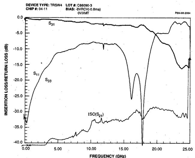
Figure 5. Small signal performance of the T/R switch (a) in Transmit mode and (b) in Receive mode.
