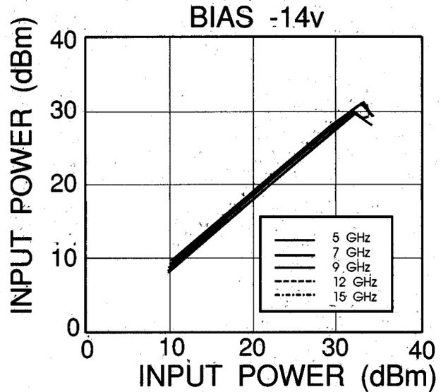
Figure 7. Power transfer curves for the T/R switch in Receive mode; output versus input power is shown.
