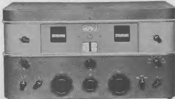
Frequency-drift compensation and tremendous usable gain makes the new AR-77 one of the most brilliant communication receivers ever hooked to an antenna. The AR-77 uses 10 tubes (5 high-gain single-ended types) and has a frequency range that extends all the way from 540 to 31,000 kc. It employs band-switching in 6 ranges with individual coils and uses a crystal filter with a 6-stage selectivity control that provides band widths from 6 kc to 80 cycles!
