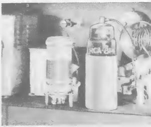
LEFT: W6ITH, top voice man, has a power amplifier that is a symbol of symmetry. Note that corresponding plate and grid leads are identical in length and as short as is mechanically possible.
