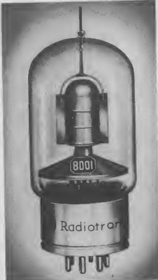
RCA-8001 takes a maximum plate input of 300 watts as high as 75 Mc with only 1.4 watts of drive—and without need for neutralization.
