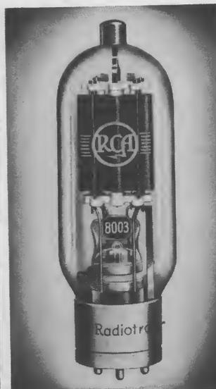
RCA-8003 delivers 250 watts at the low plate voltage of 1350 volts—up to 30 Mc. It is designed particularly to withstand high peak voltages.
