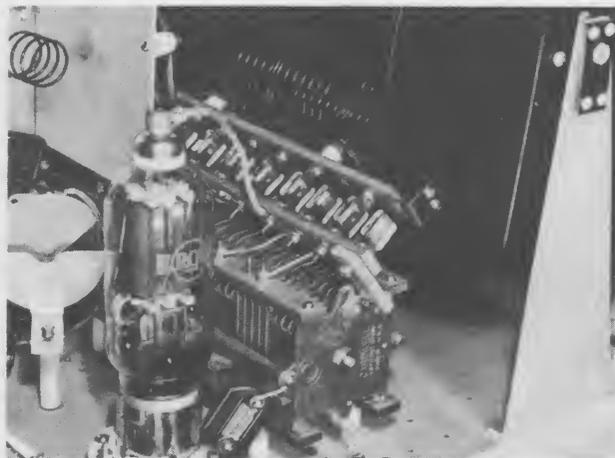
A check for \$5.00 is on the way to W6QPD of Glendale, California, for this photo of his business-like 810 final amplifier. The picture shows the coil turret which not only selects the proper inductor for the band in use, but also cuts in the proper tank capacitance. The transmitter is a band-switch affair from stem to stern. Tube complement includes an 807 as crystal or E.C. oscillator, 807 buffer, 810 final, and class B modulator 808's. Every tube in the outfit is RCA. Nice work, W6QPD!
