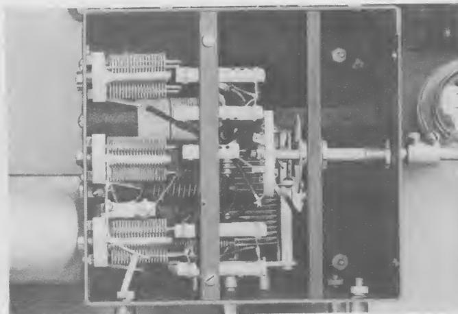
The 802 grid circuit and its associated shield enclosure is the most important unit of the VFO. The five air-padders C<sub>1</sub>, C<sub>2</sub>, C<sub>5</sub>, C<sub>7</sub> and C<sub>10</sub> and the three grid coils L<sub>1</sub>, L<sub>2</sub> and L<sub>3</sub> are mounted on the left side of the box. C<sub>13</sub> and the dial mounting arrangement are seen in the center of the box. Note the position of the five zero-coefficient condensers at the top of the assembly.
