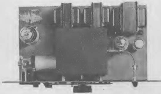
Simplicity and solid construction are key-notes of this instrument. The vital 802 control-grid circuit is enclosed in the central shield box. Note the dial-mounting arrangement and the extension of the 802 horizontally away from the box. The 807 buffer/doubler stage is rear left on the chassis, the power supply rear right.
