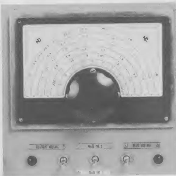
Bandspread extends from approximately  $120^\circ$  on 20 and 80 meters, to  $145^\circ$  on 10 meters. Tests show that it is practical to reset the frequency within a few hundred cycles of a marked point on 80 meters. For this reason, no provision was made for inclusion of crystals for spot-frequency operation.
