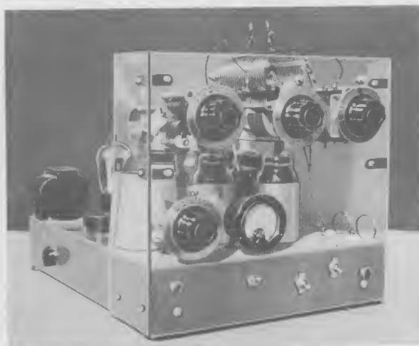
The \$5.00 prize goes to F. L. Moore, of Moffett Field, Calif., for a picture of his most novel transmitter. The rig uses a 6L6 crystal oscillator and two 807's in parallel at 120 watts input. It is built in one complete unit with self-contained power supply and an antenna coupler to match any type of radiator. No need for further details, we see right through it (!??)
