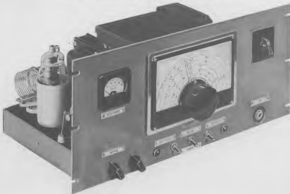
This thoroughly engineered VFO meets modern requirements for a master-control oscillator having exceptional frequency stability, break-in operation, chirpless keying, 5-band operation, high-power output, a minimum of tubes, wide bandspread on all bands, high dial-reset accuracy, and a self-contained power supply.
