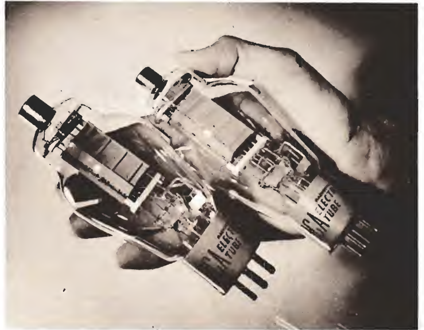
These transmitting triodes have long been the Amateurs' favorite class B modulators.
