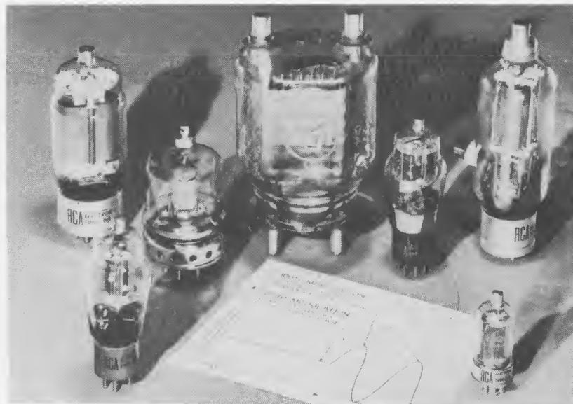
RCA power tubes have the extra safety factor required for plate-modulated service . . . ample reserve of cathode emission to satisfy modulation peaks . . . husky grid structures that permit ample drive without causing grid emission . . . high voltage insulation. Your RCA Tube Distributor has them in stock.
