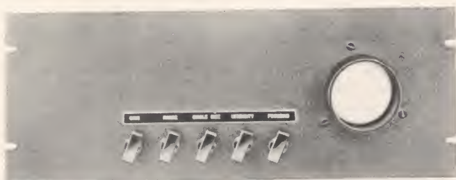
Figure 1. Panel view of the circular base line panadaptor showing position of the front controls and CR tube face.
