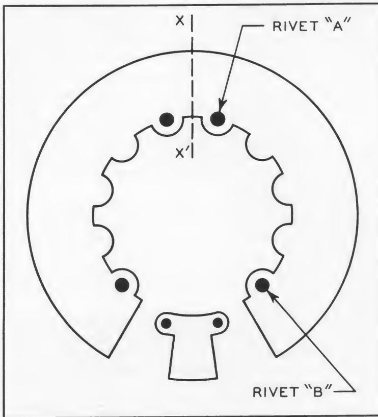
Figure 3. S1A face of switch section GG before modification. (S1B is on opposite face of this section.) Saw through switch plate along line X-X'. Drill rivet "A" until it is loose, but do not remove. Drill rivet "B" and remove. Remove portion of switch plate to right of line X-X'. Crimp rivet "A" tight again. (Rivet "A" helps secure S1B.)
