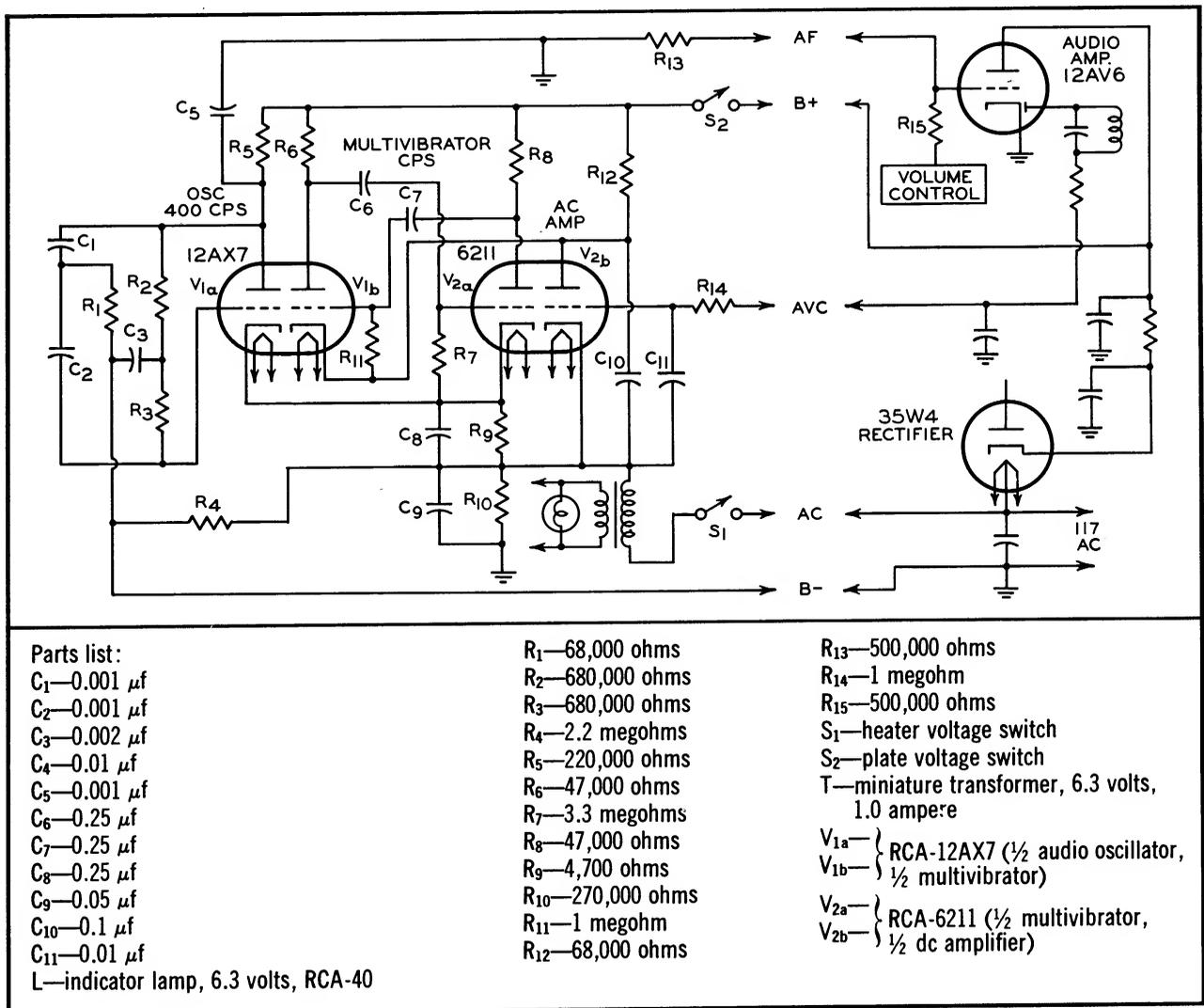
Schematic and parts list for automatic Conelrad unit.
