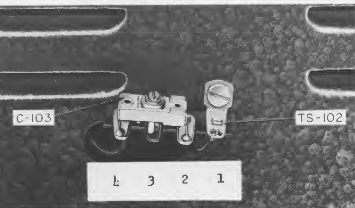
Figure 3: The four-lug terminal strip (TS-102) is mounted on the rear of the case.
