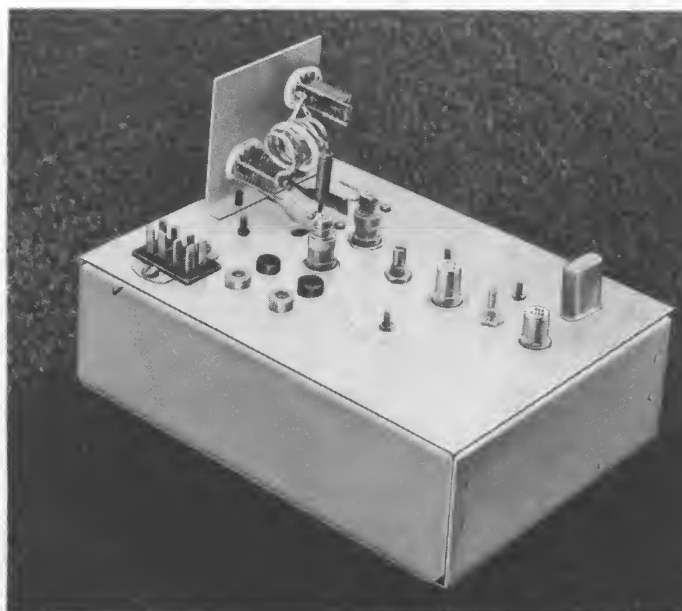
Top view of W2OKO's two-meter transmitter designed around two RCA-7586 nuvistor triodes and a pair of RCA-7587 nuvistor tetrodes.
