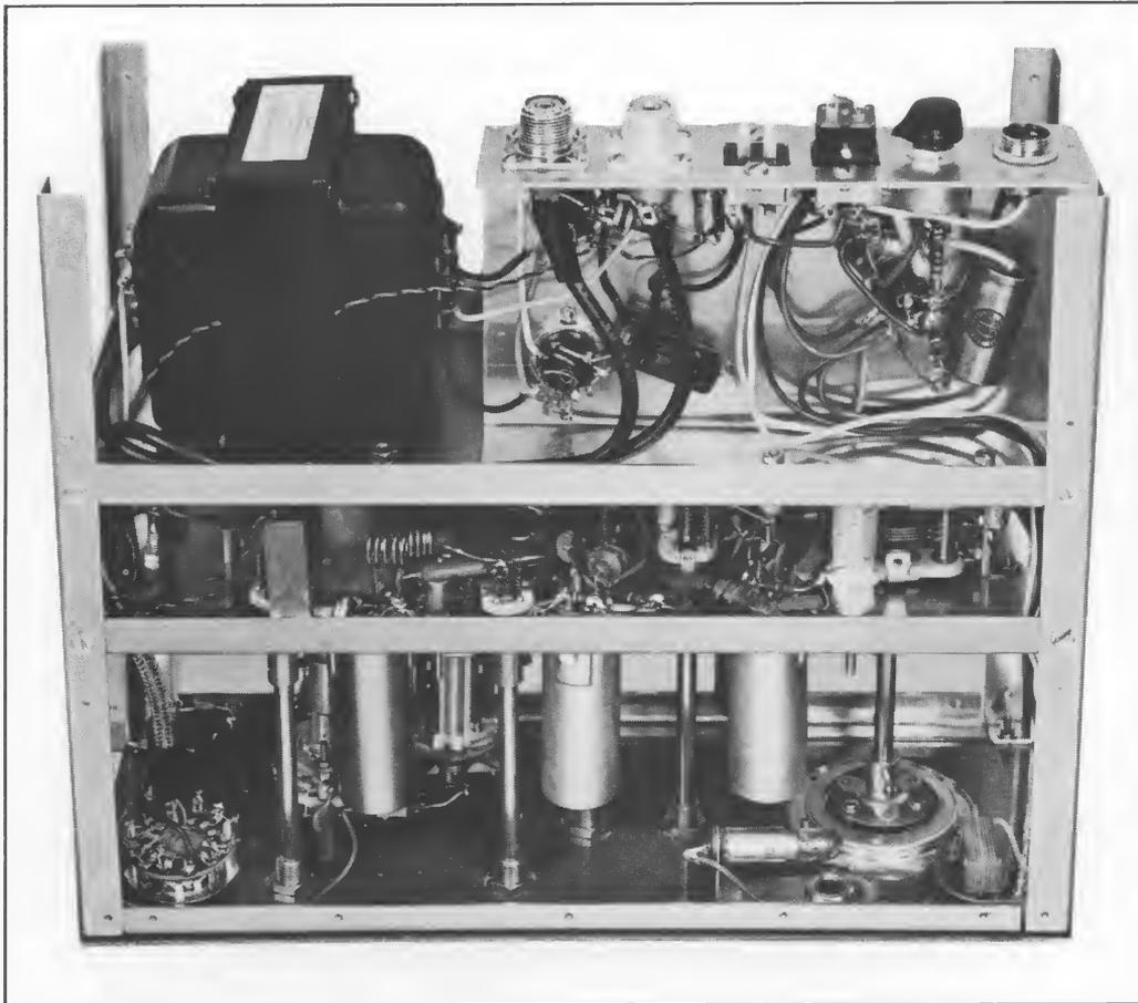
Bottom view showing modulator construction and rf section.
