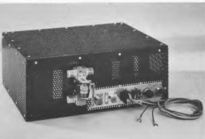
Rear view of new mobile transmitter showing antenna relay, microphone connector, and power connectors.
