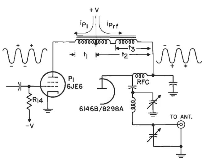
Figure 1: Autotransformer connections showing details of step-up configuration.
