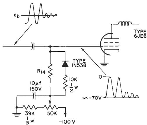
Figure 5: Insertion and operation of clamp diode.
