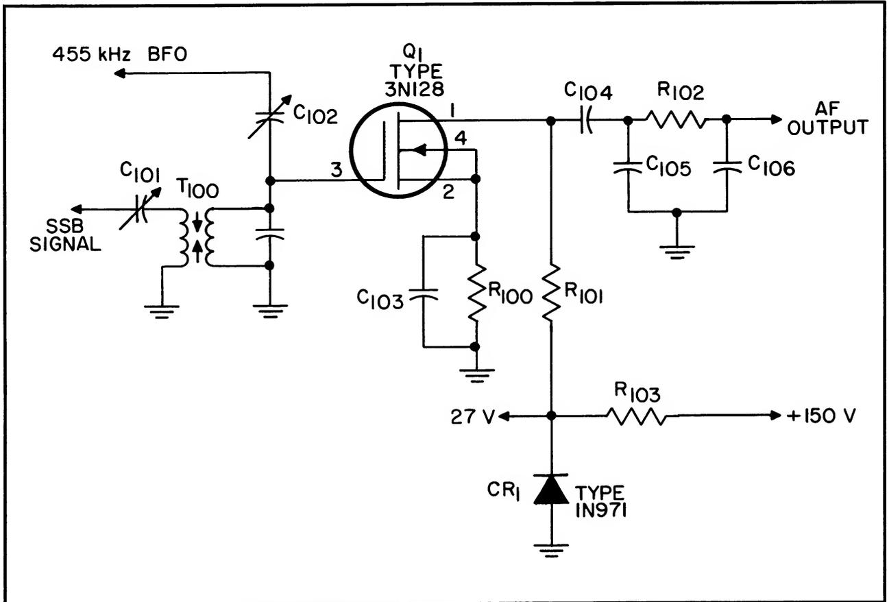
Figure 3: Schematic diagram of product detector.
