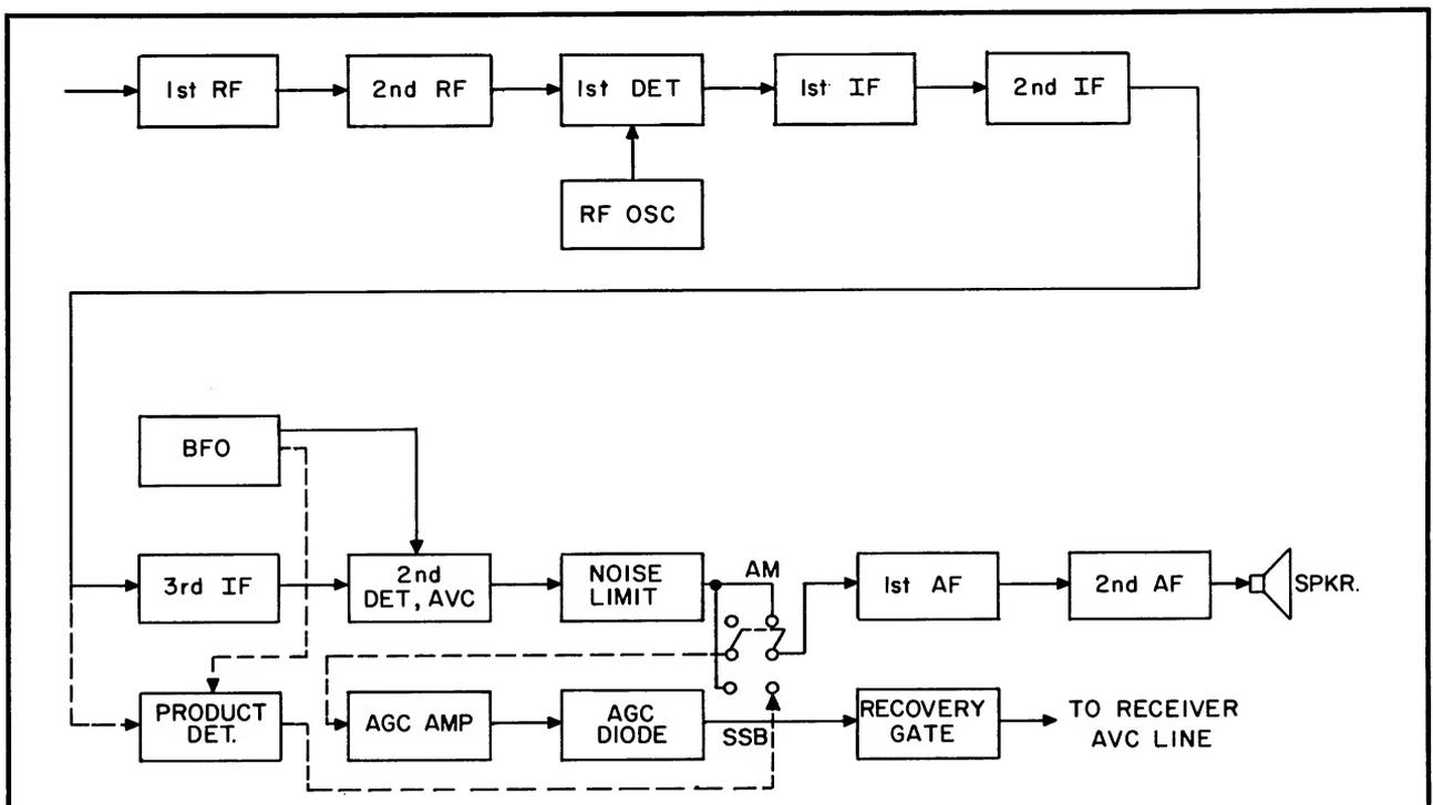
Figure 2: Block diagram of a typical general-purpose communications receiver showing additions (dashed lines) of product detector and AGC system.
