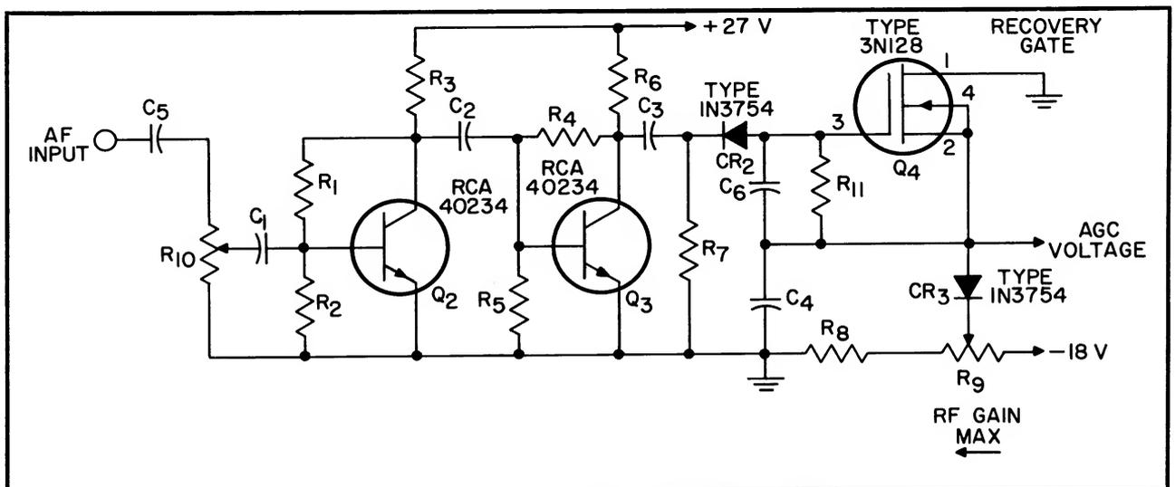
Figure 4: Schematic diagram of AGC system.
