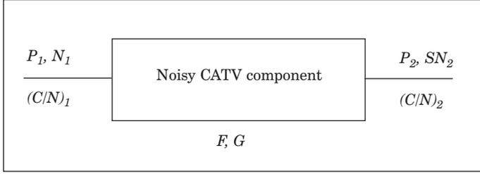
■ **Figure 6. Noisy component at a general position in the CATV cascade.**
