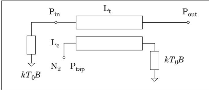
■ Figure 3. Lossless directional coupler model.
