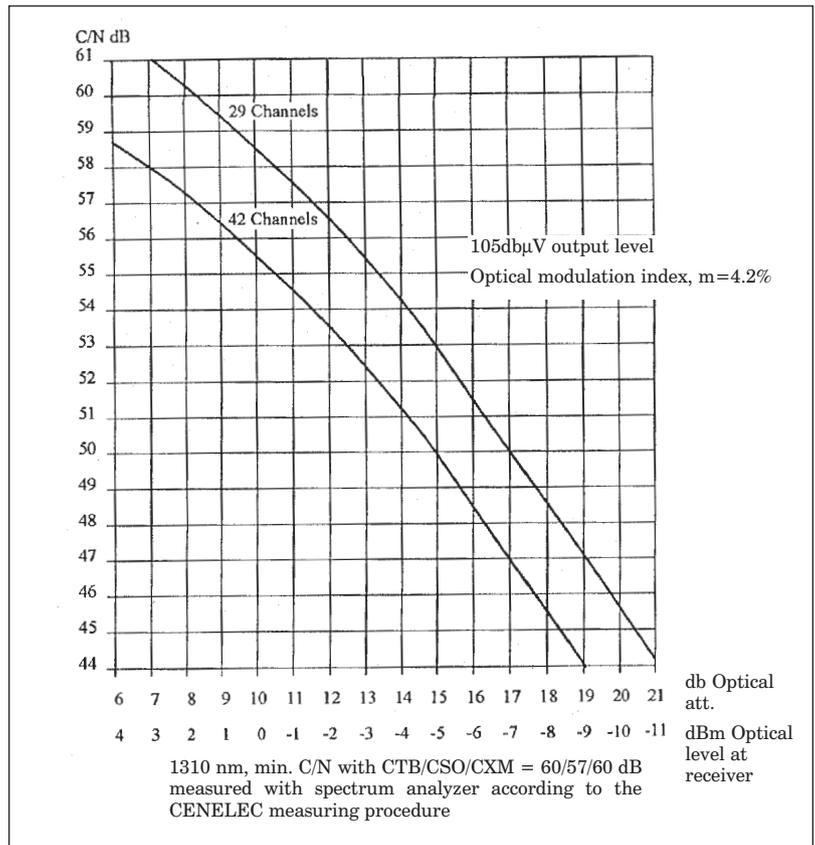
■ Figure 1.  $C/N_{OTX}$  [dB] versus  $P_{in}$  [dBm] plot (transmitter 90019, receiver 90060, courtesy ARCODAN company.)
