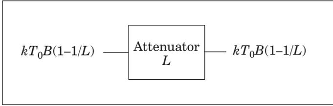
■ Figure 2. Attenuator thermal noise radiation.
