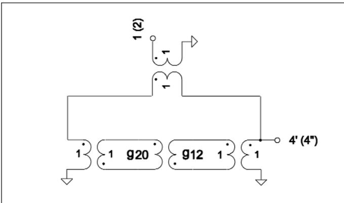
▲ **Figure 7.** Simplified circuit Figure 6 when length of each line is 90 degrees.
