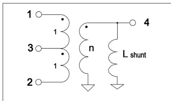
▲ **Figure 1. Schematic model of typical hybrid at lower frequencies.**
