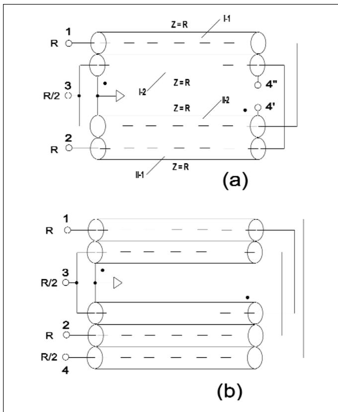
▲ **Figure 2. Broadband transmission line with single shunt inductance and (a) balanced differential port; (b) all ports unbalanced. Two dots indicate uni-polarity ends of lines.**
