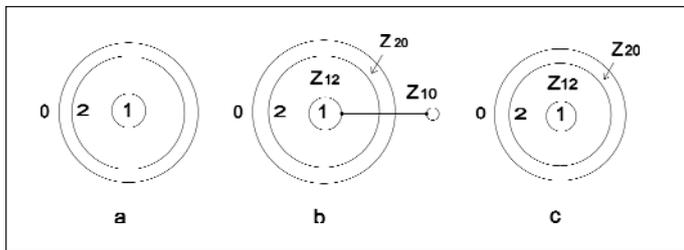
▲ **Figure 8. Possible realizations of line II in circuit Fig.4: (a) with minimum conductors; (b) with extra line that realizes coupling between lines; (c) simplified solution that introduces small mismatch.**
