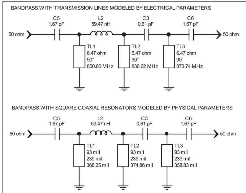
▲ **Figure 5. An 825 to 849 MHz bandpass filter with shunt L-C resonators replaced with equivalent electrical transmission line elements (top) and with physical models for square coax specified by the inner conductor diameter, side dimensions and length in mils (bottom). The physical parameters given are for the Trans-Tech 9000 Series small profile (SP) coaxial resonators.**
