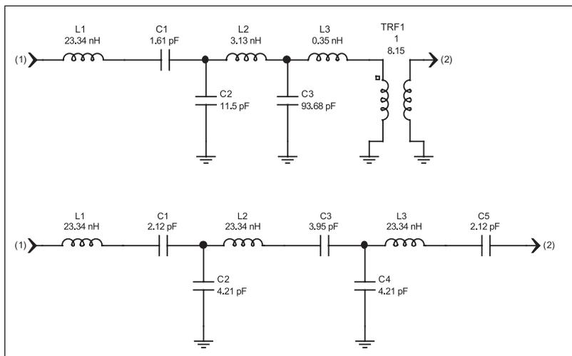
▲ **Figure 7.** A 3-section 700 to 1,000 MHz bandpass filter designed using direct synthesis (top) and then transformed to a pure series-resonator configuration by applying shunt Norton transforms to C2 to place a capacitor in series with L2 and to C4 to place a capacitor in series with L3.
