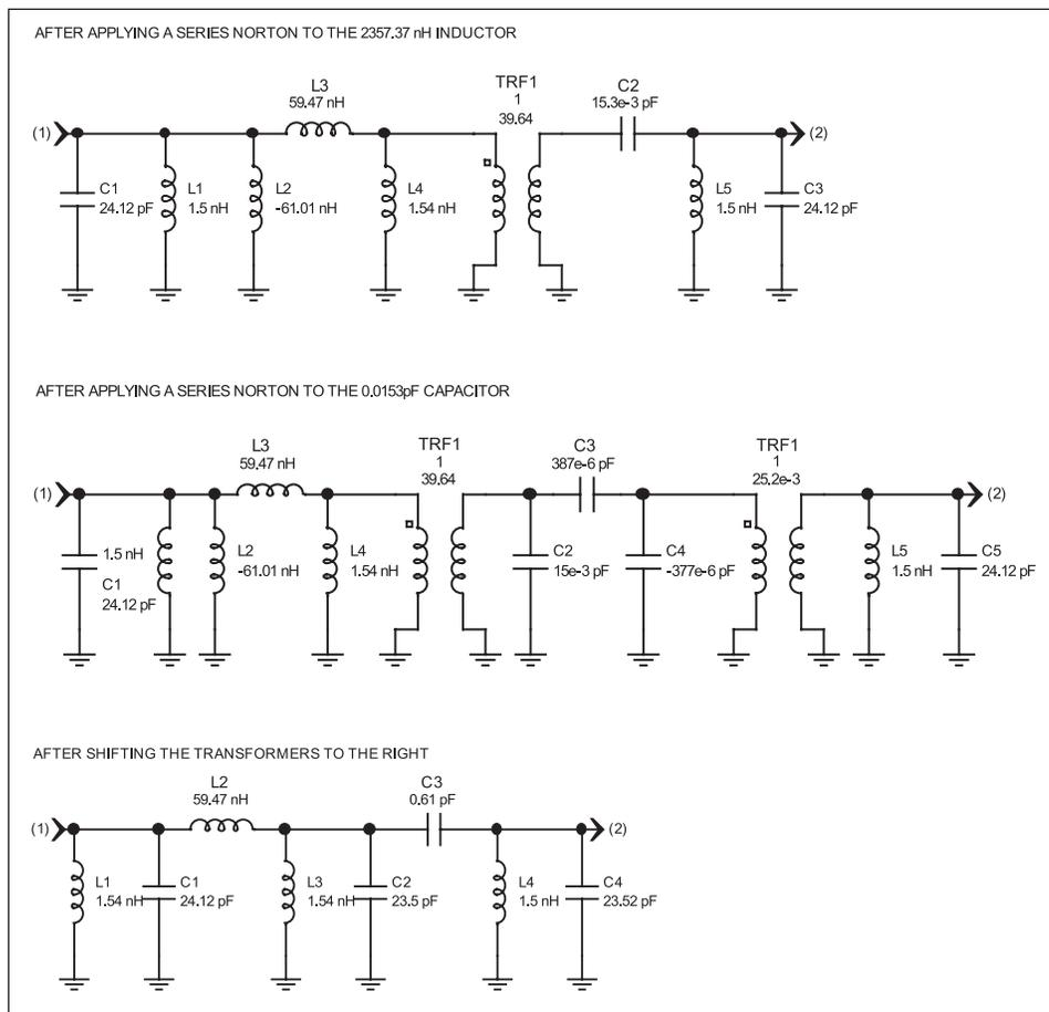
▲ **Figure 2.** Schematic after applying the series Norton transform to L2 in Figure 1 with  $N = 39.64$  (top schematic), after applying the series Norton to C2 in Figure 1 with  $N = 1/39.64 = 0.02523$  (middle schematic) and after shifting the transformers to the right (bottom schematic).
