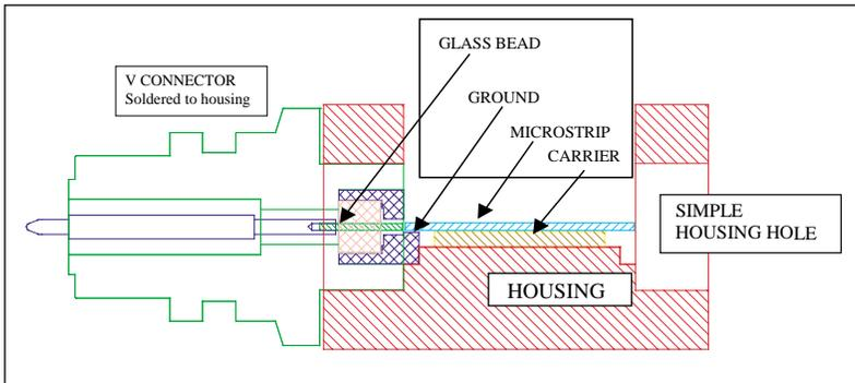
▲ Figure 15. Connector for substrates on carriers.
