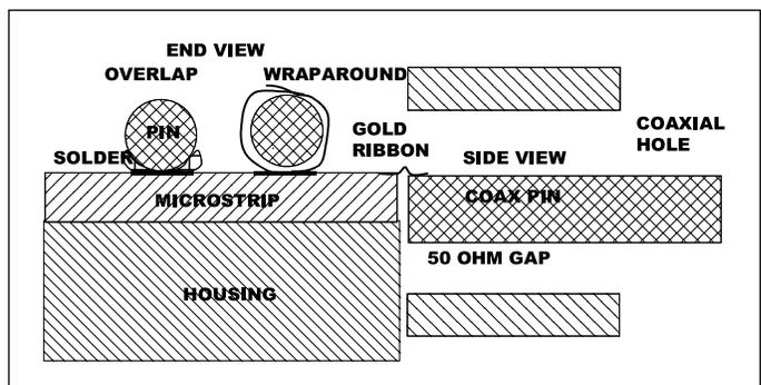
▲ Figure 3. Coax pin to microstrip connections.
