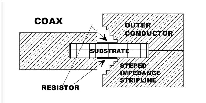
▲ Figure 6. Planar resistor coaxial termination.
