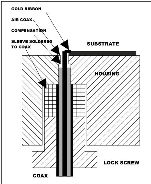
▲ Figure 4. Orthogonal connection.
