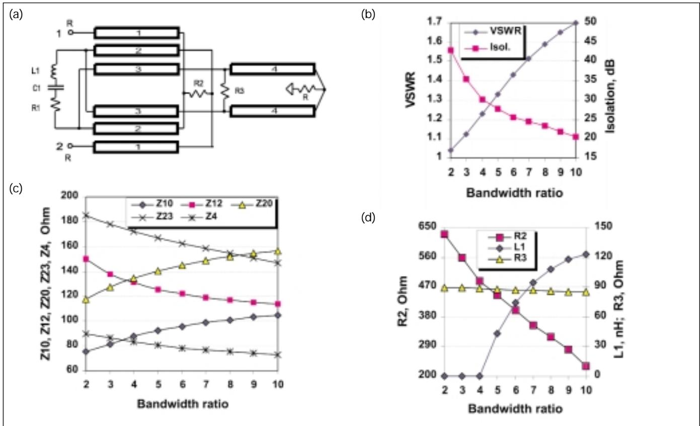
▲ Figure 12. (a) Two-section coupled-line power combiner and (b-d) its characteristics.
