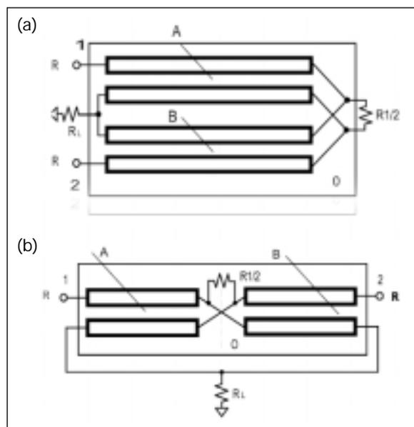
▲ Figure 1. (a) Two-way, two-conductor coupled transmission line power combiner; (b) with vertical line of symmetry.
