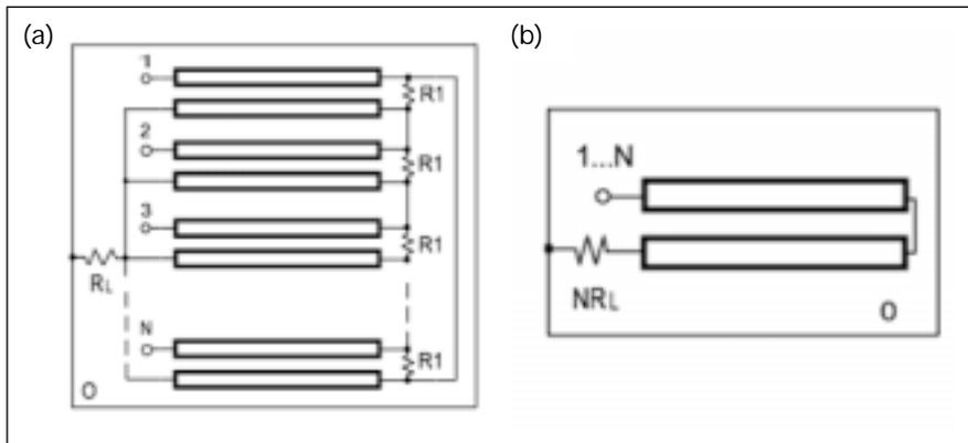
▲ Figure 4. (a) Single-section N-way combiner with two-conductor coupled lines; (b) in-phase decomposition circuit.
