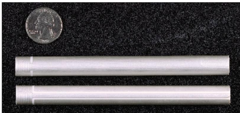
▲ Figure 6. Photograph of the cylindrical slot antennas fabricated on 1.27 cm diameter alumina rods. The upper image shows the shorted ends of the slot on the back side of the antenna. The lower image shows the cylindrical coupled slot feedline.
