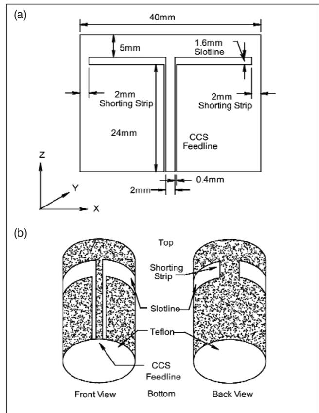
▲ **Figure 1. Cylindrical slot line antenna on PTFE: (a) two-dimensional view illustrating line and slot widths; (b) three-dimensional view with metal regions shaded (SMA connector not shown).**
