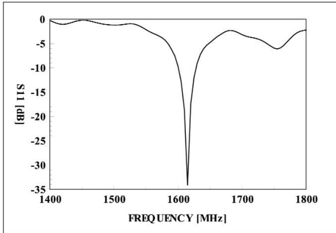
▲ **Figure 7.** Measured input reflection coefficient ( $S_{11}$ ) for the cylindrical slot antenna on alumina.
