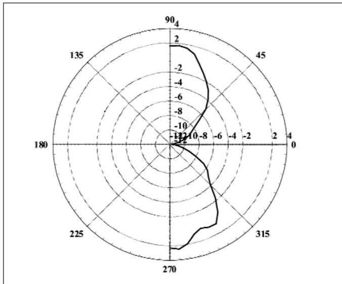
▲ **Figure 9.** Measured E-plane gain pattern for the cylindrical slot antenna on alumina. The top of the cylindrical alumina rod corresponds to 0 degrees.
