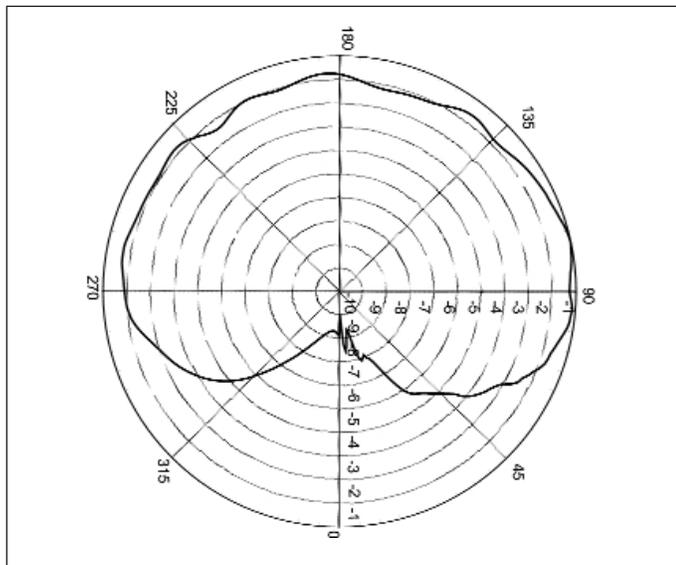
▲ Figure 4. H-plane slot antenna radiation pattern with CCS feedline side of antenna referenced to 0 degrees.
