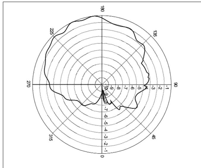
▲ Figure 5. H-plane folded slot antenna radiation pattern with CCS feedline side of antenna referenced to 0 degrees.
