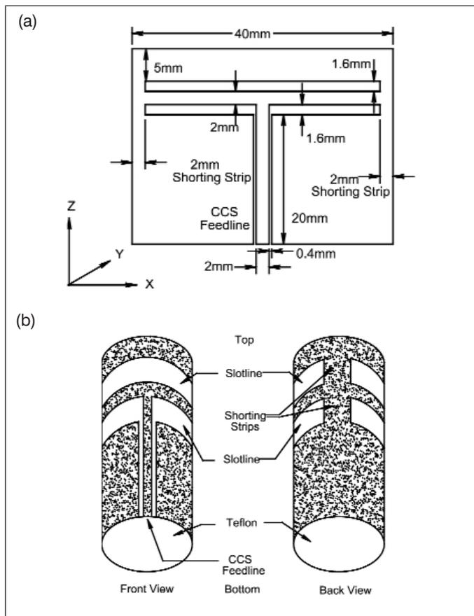
▲ **Figure 2. Cylindrical folded slot line antenna on PTFE: (a) two-dimensional view illustrating line and slot widths; (b) three-dimensional view with metal regions shaded (SMA connector not shown).**
