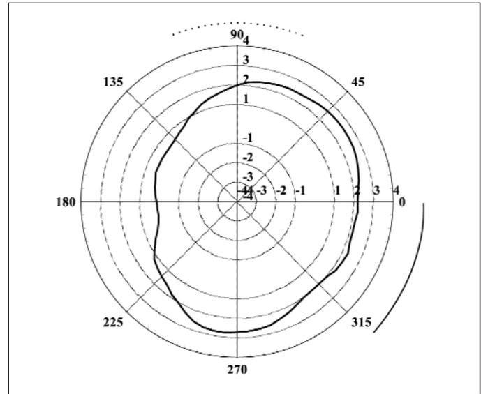
▲ **Figure 8.** Measured H-plane gain pattern for the cylindrical slot antenna on alumina. The feedline location is indicated by the dashed line centered around 90 degrees, while the shorted slot section is indicated by the solid line centered around 348 degrees.
