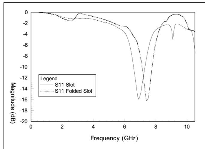
▲ **Figure 3. Measured response of the antennas on PTFE with a 52-ohm (slot) and 40-ohm (folded slot)  $\lambda_g/4$  impedance transformer.**
