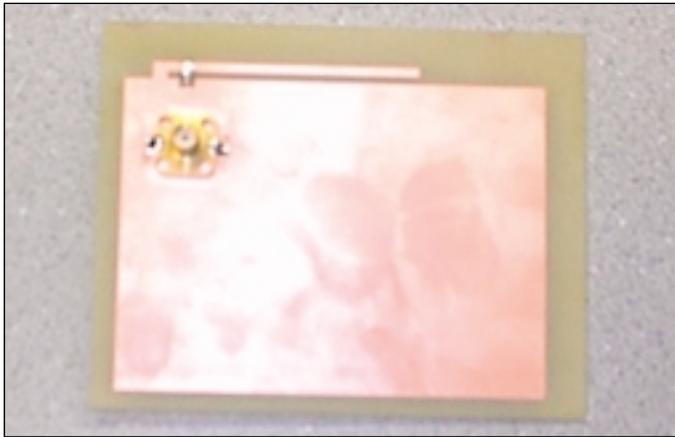
▲ Figure 12. Experimental layout of an IIFA.
