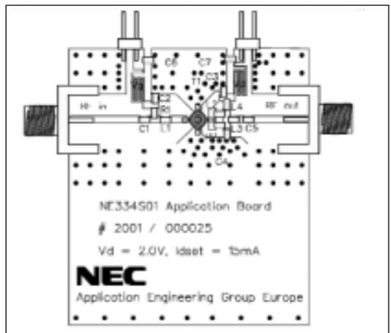
▲ Figure 10. Layout and component placement.
