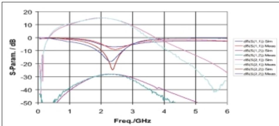
▲ Figure 6. S-parameters (simulation versus measurement) up to 6 GHz.
