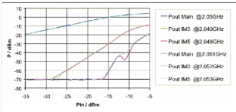
▲ Figure 8. Intermodulation characteristic.
