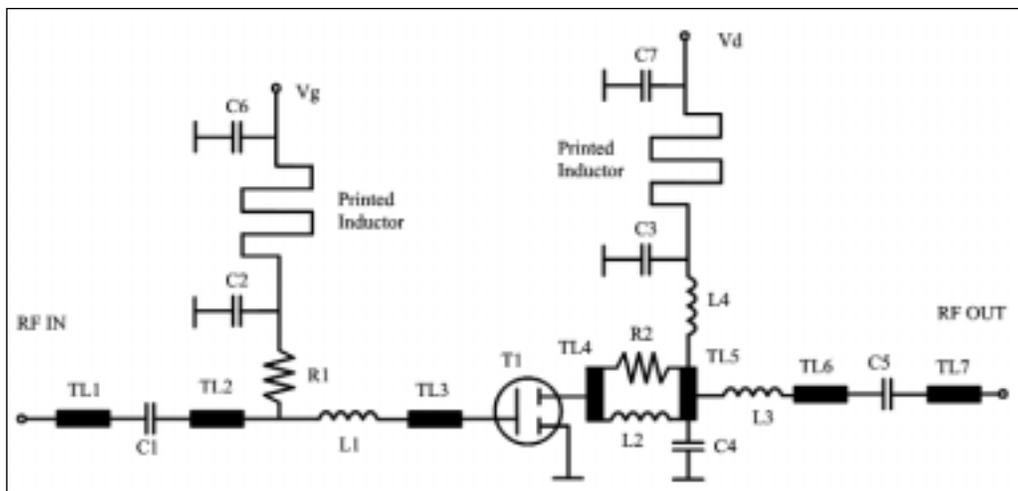
▲ Figure 3. Schematic of the low-noise amplifier.
