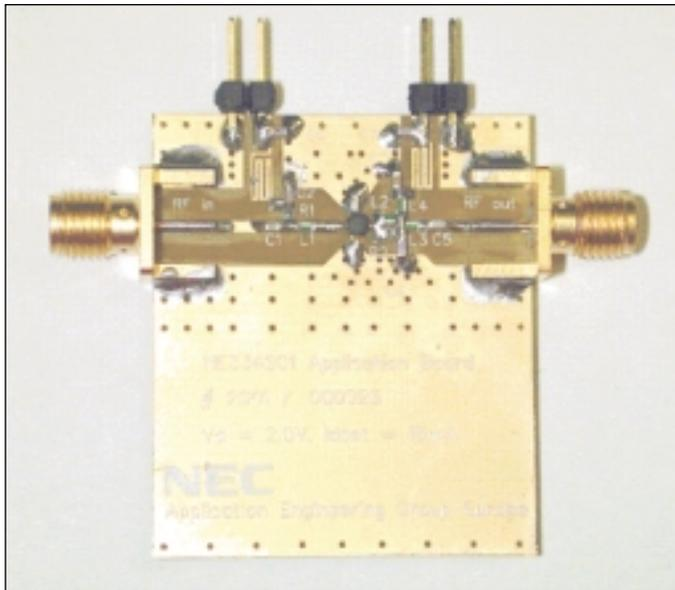
▲ Figure 2. Application board of the low-noise amplifier.
