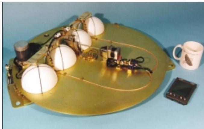
▲ Figure 3. A Luneberg lens cut in half and placed on a ground plane can duplicate the performance of a full spherical lens at half the height, making it ideal for airborne applications which would require a low profile to reduce wind drag.
