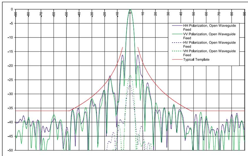
▲ Figure 2. Antenna pattern of a six-layer, 16-inch diameter Luneberg lens.
