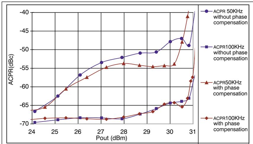
▲ Figure 3. Measured ACPR characteristics of the PA, with and without phase compensation.
