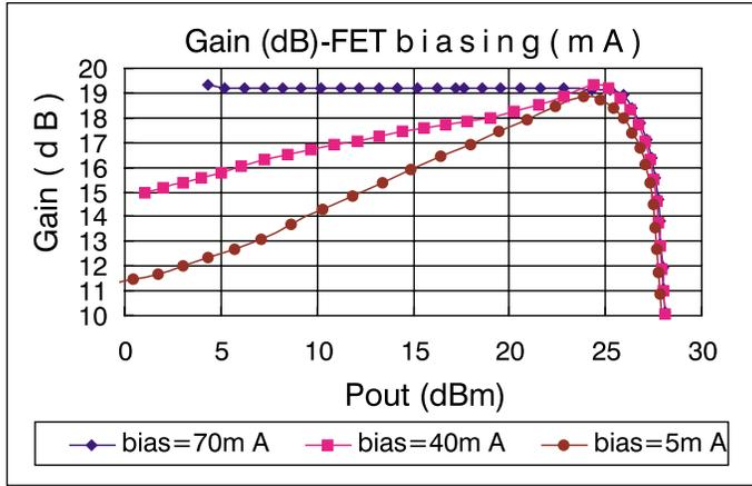
▲ Figure 1. Measured gain and bias characteristics of a FET.
