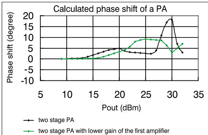
▲ Figure 2. Calculated phase shift of a two-stage PA.
