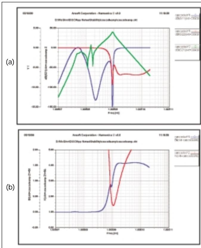
▲ Figure 7. (a) Small-signal and (b) linear stability criteria of the two-stage amplifier.
