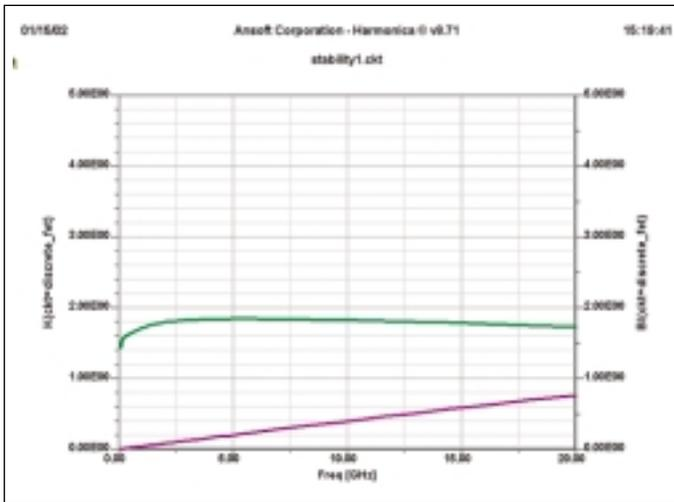
▲ Figure 2. The K1 and B1 of the example transistor.
