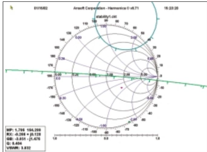
▲ Figure 3.  $S_{11}$ ,  $S_{22}$  and stability circles at 880 MHz.
