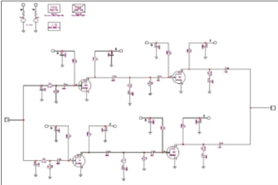
▲ Figure 6. Sample amplifier topology composed of dual two-stage cascaded amplifiers in parallel.
