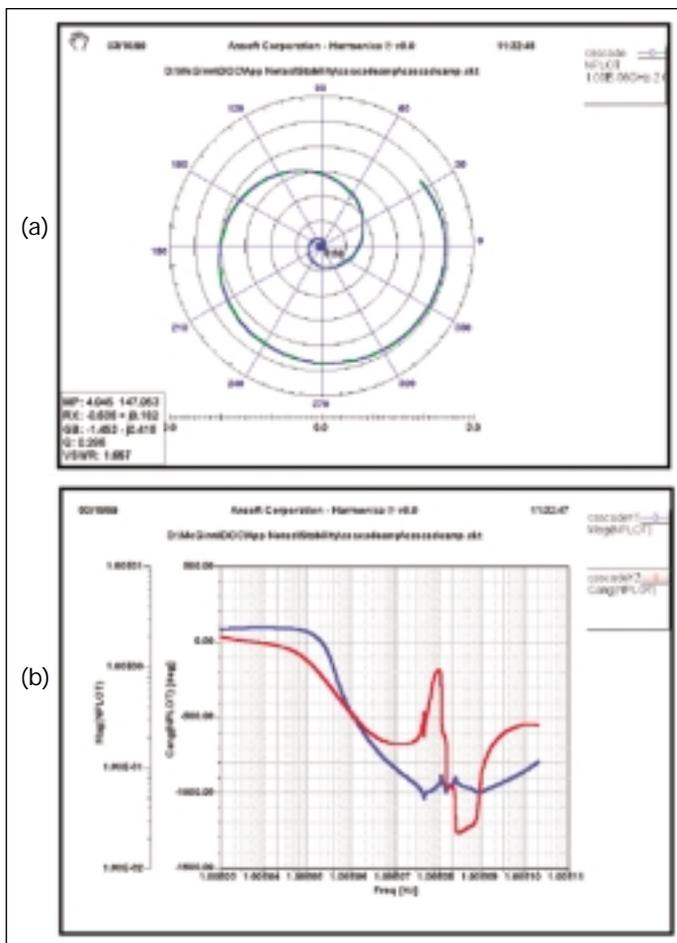
▲ Figure 8. (a) Polar Nyquist plot of an unstable two-stage amplifier and (b) a magnitude/cumulative angle Nyquist plot of the amplifier.
