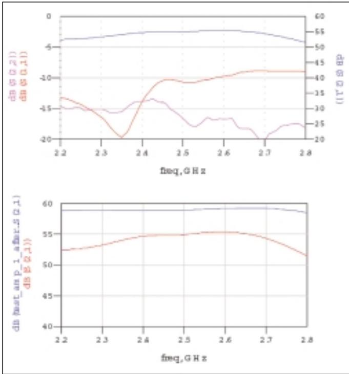
▲ Figure 4. S-parameters simulation and experimental results of the power amplifier.
