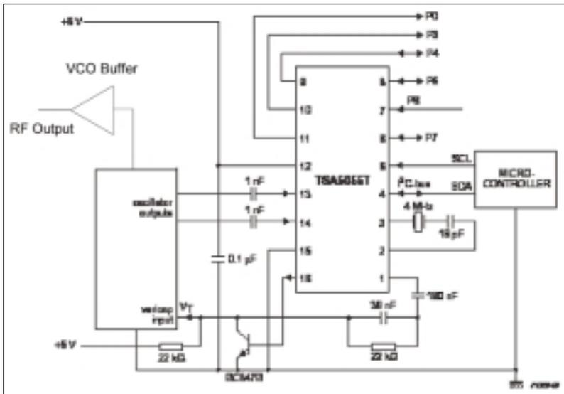
▲ Figure 6. Schematic of the phase-locked oscillator.
