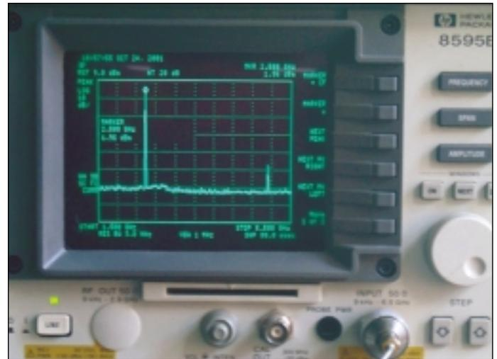
▲ Figure 5. Spectrum analyzer display of the output spectrum of the power amplifier.
