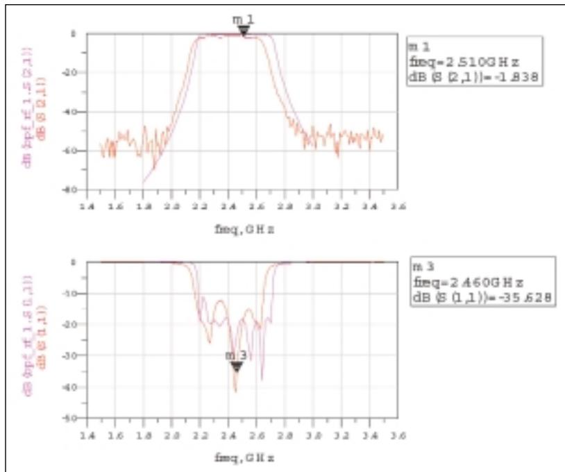
▲ Figure 3. Simulation and experimental results of the stripline filter.
