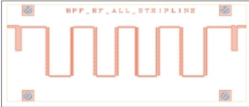
▲ Figure 2. Layout of the stripline bandpass filter.
