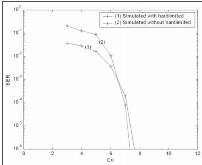
▲ Figure 9. Simulated BER with and without the hard-limited for CCI center frequency of  $f_c - 250$  kHz.
