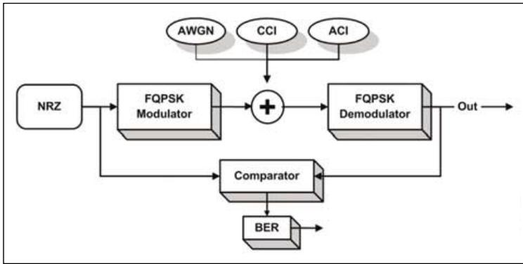
▲ Figure 1. Simulation scheme without the hard-limited filter.
