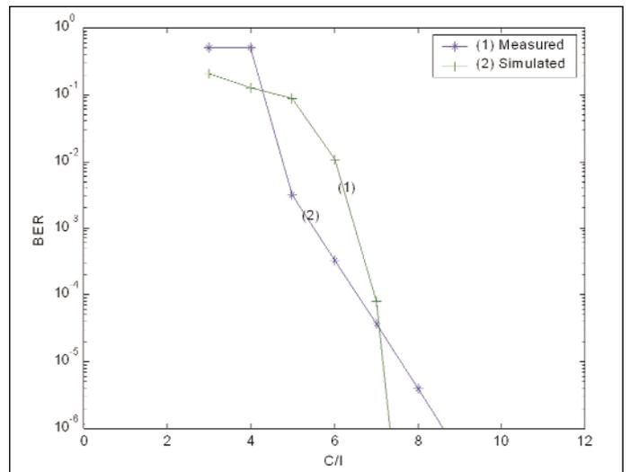
▲ Figure 6. Comparison of the simulated and measured results for CCI center frequency =  $f_c - 250$  kHz without the hard-limited filter.
