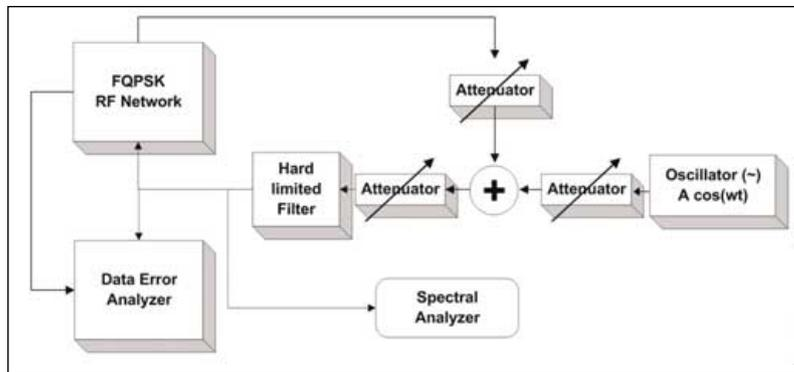
▲ Figure 8. Measurement scheme with the hard-limited filter.
