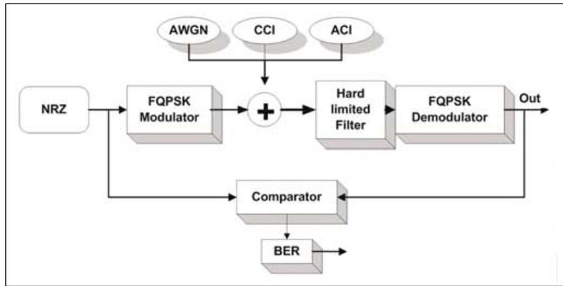
▲ Figure 7. Simulation scheme with the hard-limited filter.
