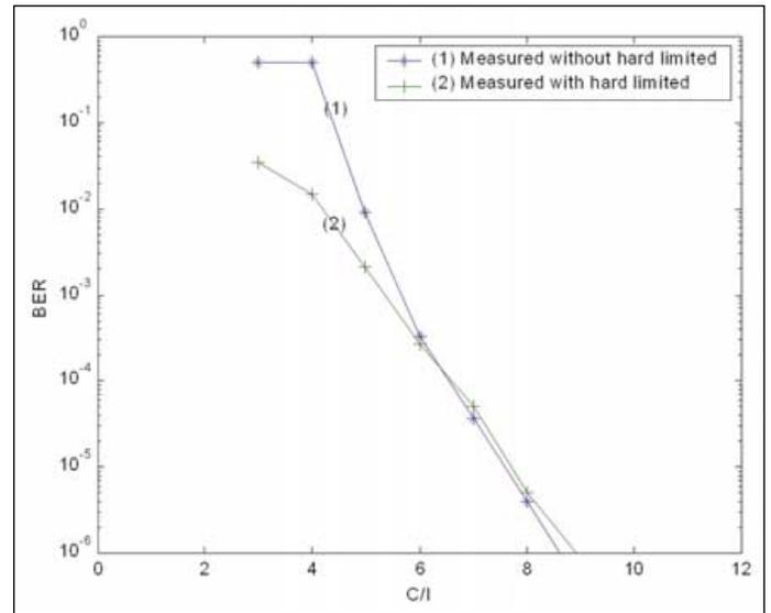
▲ Figure 10. Measured BER with and without the hard limited for CCI center frequency of  $f_c - 250$  kHz.
