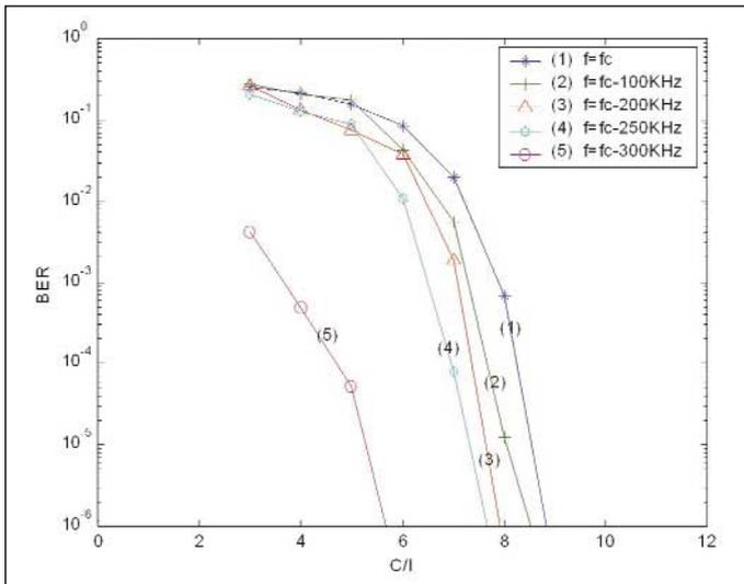
▲ Figure 2. Simulation results for different CCI center frequencies without the hard-limited filter.
