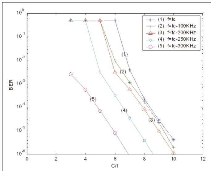
▲ Figure 5. Measurement results for different CCI center frequencies without the hard-limited filter.
