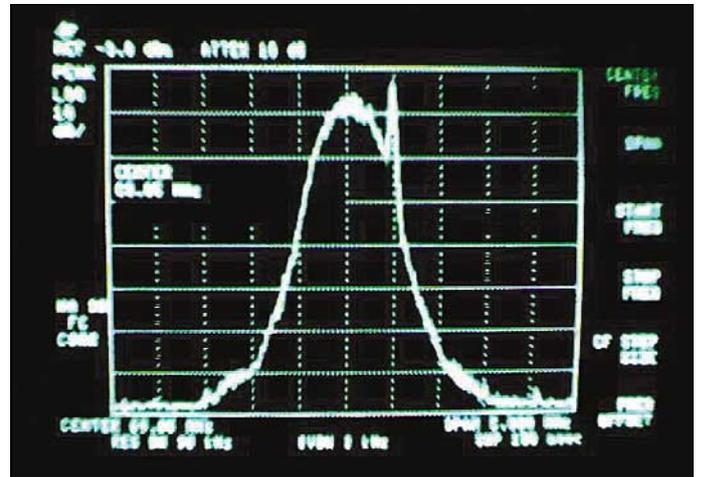
▲ Figure 4. FQPSK-B spectrum with CCI at  $f = f_c + 450$  kHz, 1 Mb/s and  $f_c = 70$  MHz.
