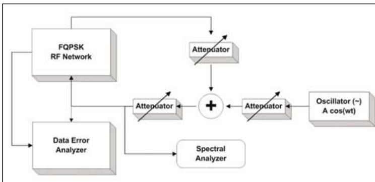
▲ Figure 3. Measurement scheme without the hard-limited filter.
