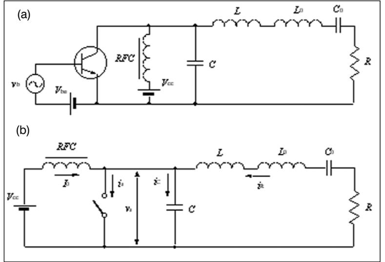
▲ Figure 3. Equivalent circuits of Class E power amplifiers with series  $LC$ -filter.
