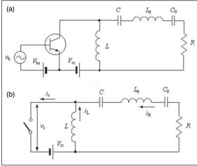
▲ **Figure 11. Class E power amplifiers (a) with shunt inductance and (b) equivalent power amplifier circuit.**
