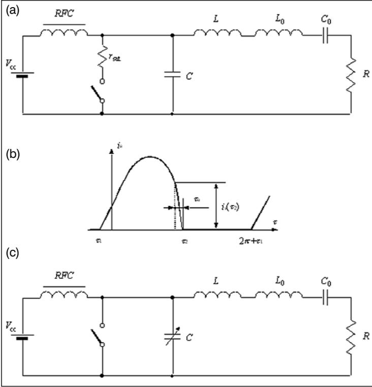
▲ **Figure 6. Equivalent Class E loading networks (a) with saturation resistance, (b) current waveform with finite time delay and (c) nonlinear capacitance.**
