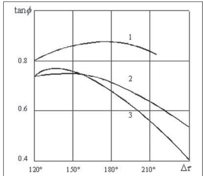
▲ Figure 10. Overall loading network phase angle for Class E tuned power amplifiers with shunt capacitance and a parallel circuit.
