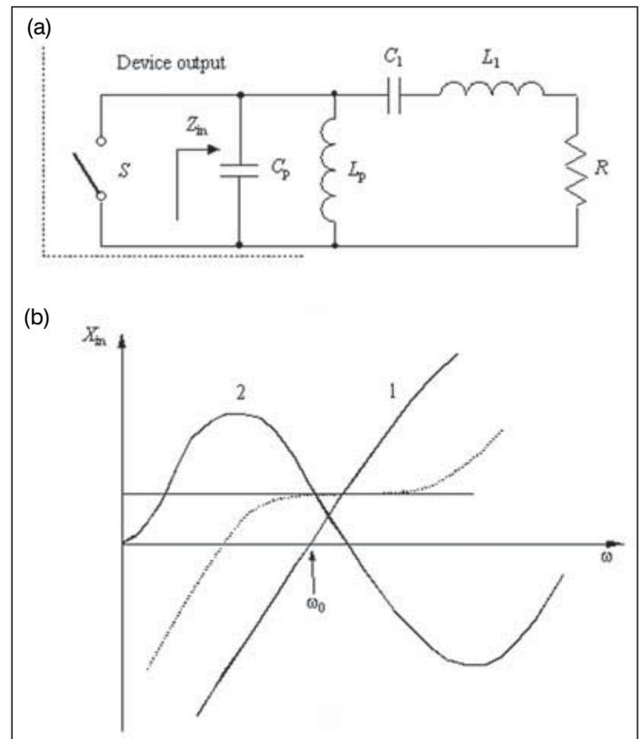
▲ **Figure 13. Single reactance compensation circuit and reactance compensation principle.**
