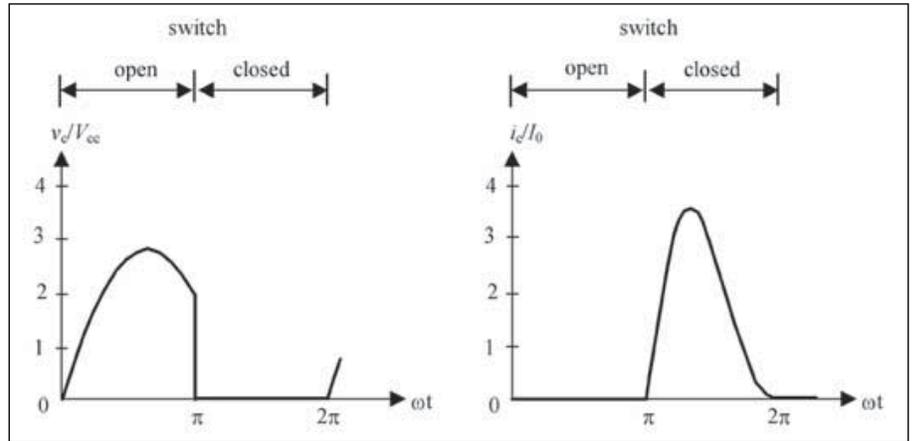
▲ **Figure 12. Voltage and current waveforms for optimum Class E operation with shunt inductance.**
