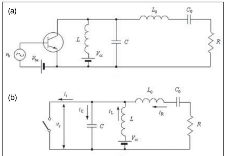
▲ Figure 7. Equivalent circuits of Class E power amplifiers with a parallel circuit.
