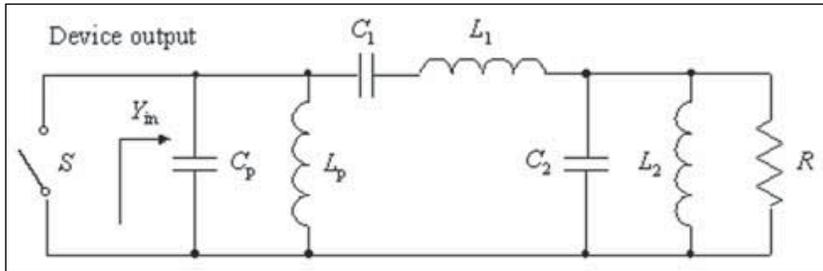
▲ Figure 14. Double-resonant reactance compensation circuit.
