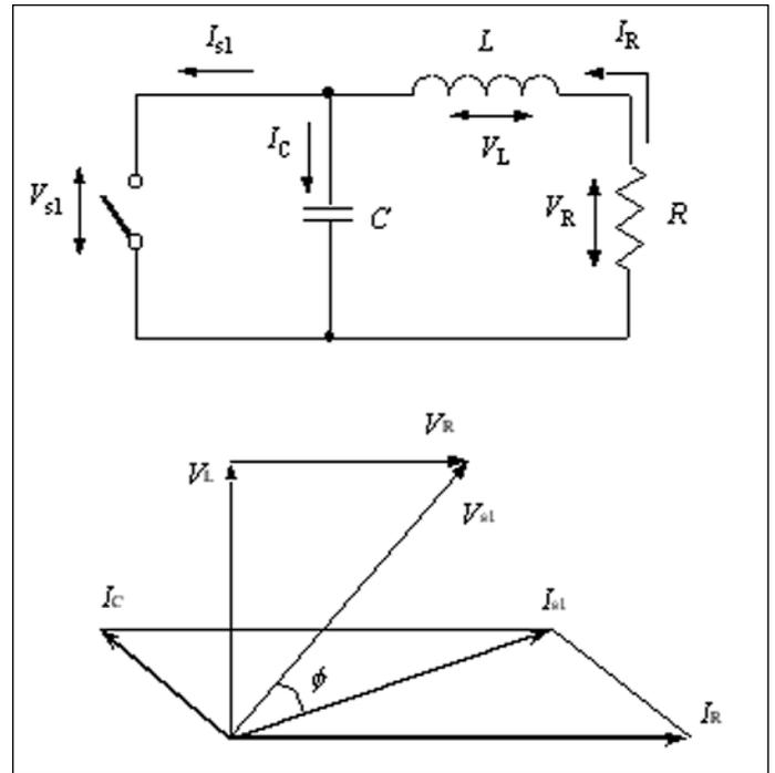
▲ Figure 5. Fundamental voltage and current phasors for equivalent circuit diagram corresponding to Class E power amplifier with shunt capacitance.
