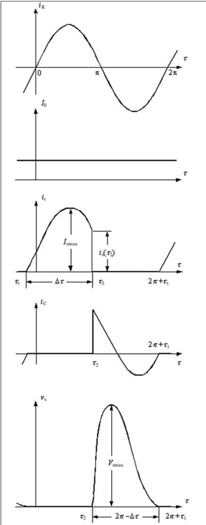
▲ Figure 4. Voltage and current waveforms for optimum Class E operation with shunt capacitance.
