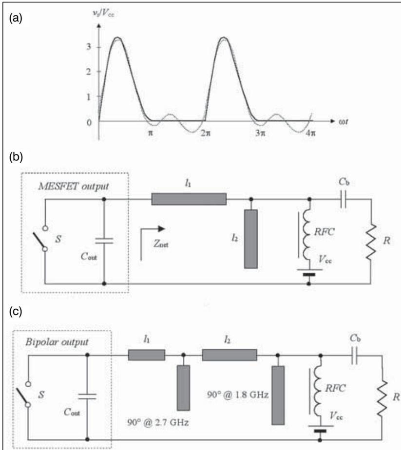
▲ Figure 15. Two-harmonic voltage waveform and equivalent circuits of Class E power amplifiers with transmission lines.
