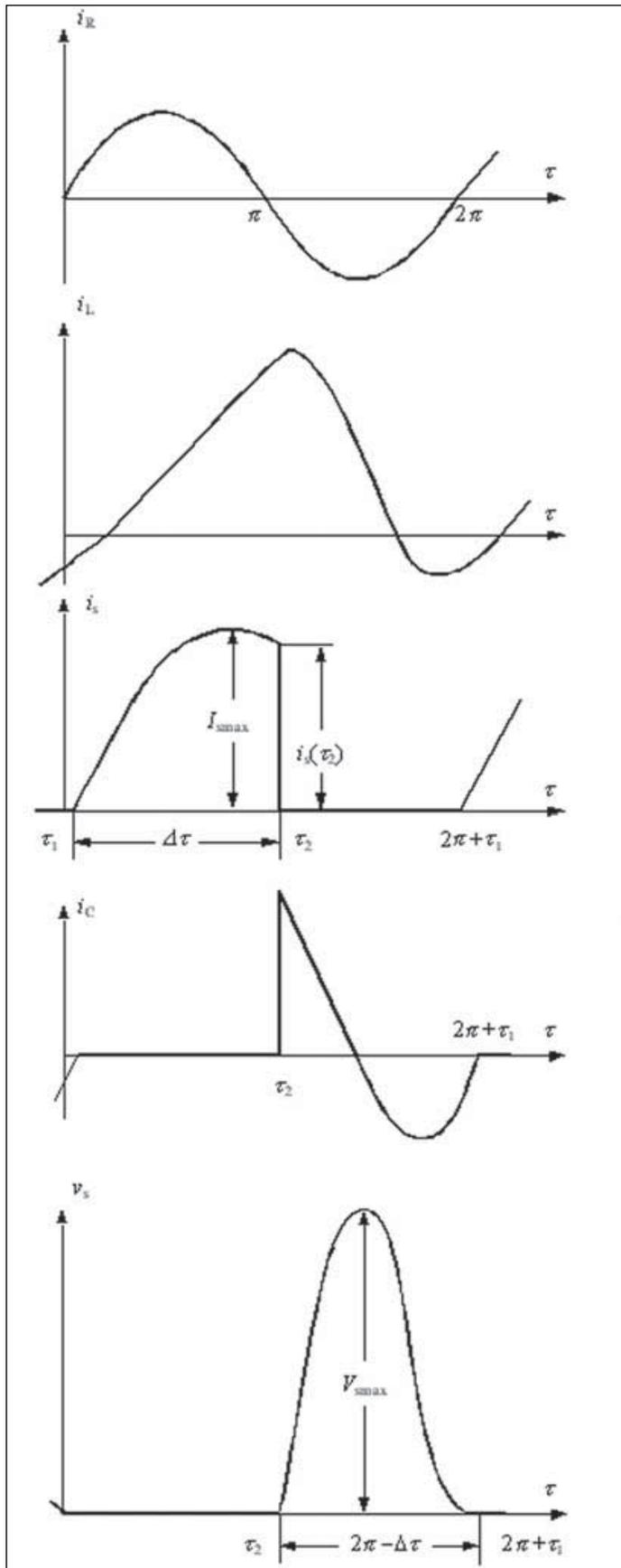
▲ Figure 9. Voltage and current waveforms for optimum Class E operation with a parallel circuit.
