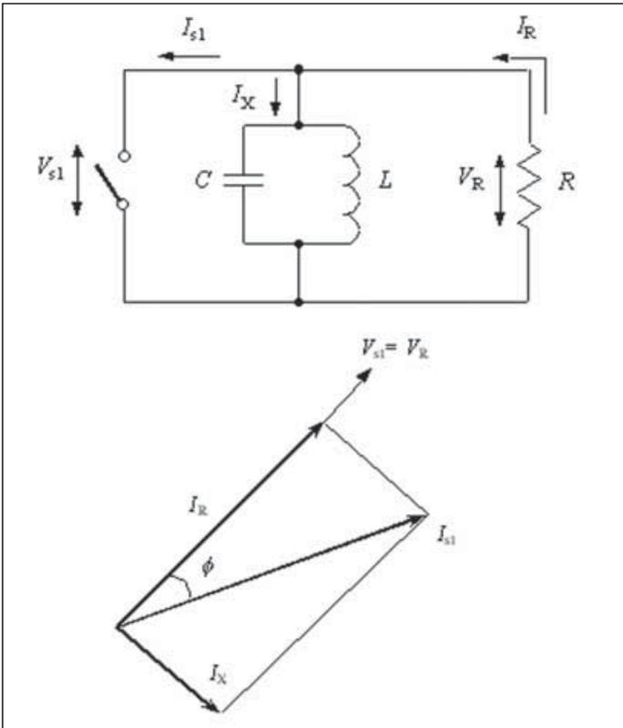
▲ **Figure 8. Phasor diagram corresponding to a Class E power amplifier with a parallel circuit.**
