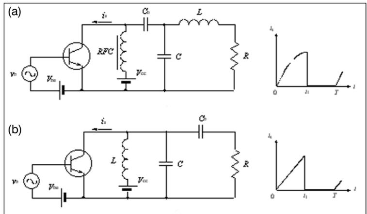
▲ Figure 1. Single-ended switching power amplifiers with (a) shunt capacitance and series inductance and (b) parallel circuit.
