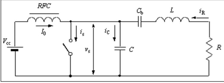
▲ **Figure 2. Basic equivalent circuit of Class E power amplifier with one inductance and one capacitance.**
