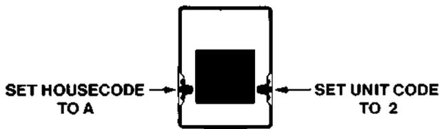
Pressing the top "2" button (for unit code 2) on the Controller will turn on the appliance. Pressing the bottom "2" will turn the appliance off. Refer to Appendix B, Troubleshooting, if this does not happen.
