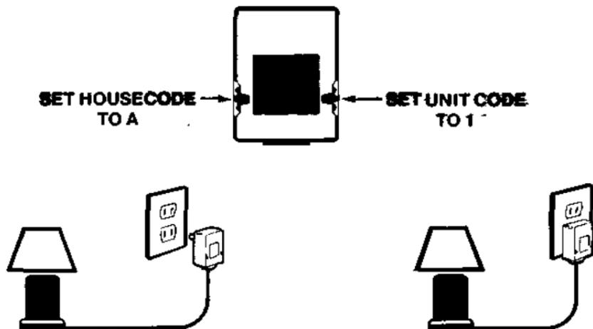
Press the top "1" button (for unit code 1) on the Controller and the lamp will go on. Press the bottom "1" button (for unit code 1) and the lamp will go off. Refer to Appendix B, Troubleshooting, if this does not happen.
