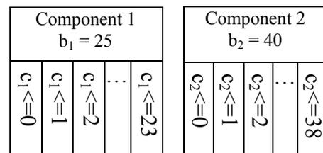
**Figure 3: An illustration of a 2-component bitmap index.**
