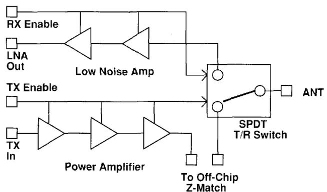
Fig. 1. Antenna Interface ASIC Block Diagram
