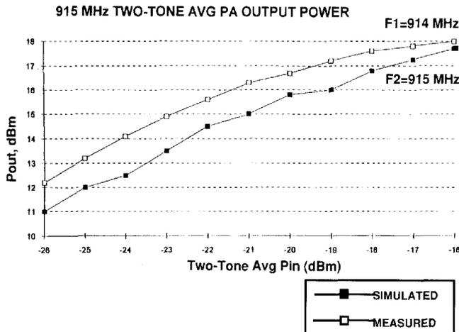
Figure 9. Simulated versus measured output power.
