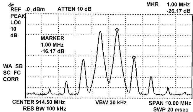
Figure 11. Measured IM3, Pin = -21 dBm Two-Tone Avg.
