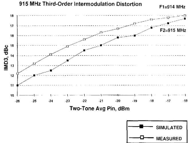
Figure 10. Simulated versus Measured Third-Order IMD.
