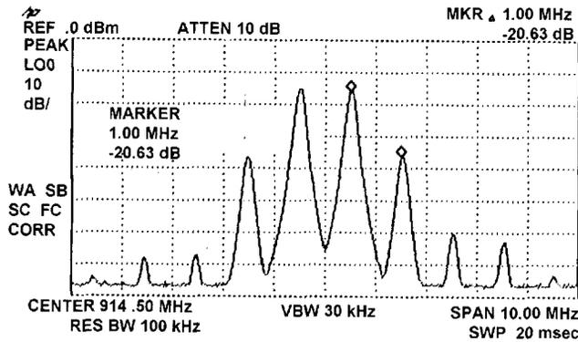
Figure 8. Measured IM3, Pin = -19 dBm Two-Tone Avg.
