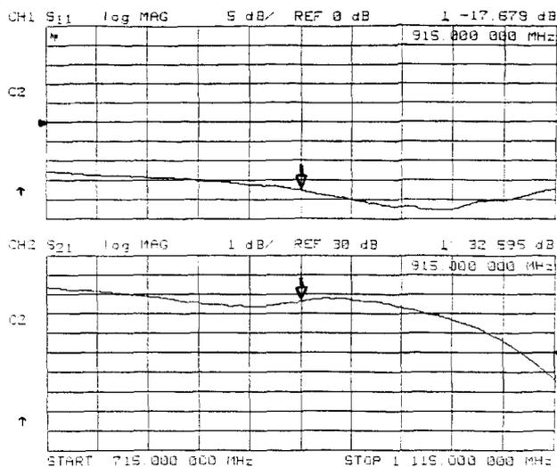
Figure 4. Measured IRL and Large-Signal Gain.
