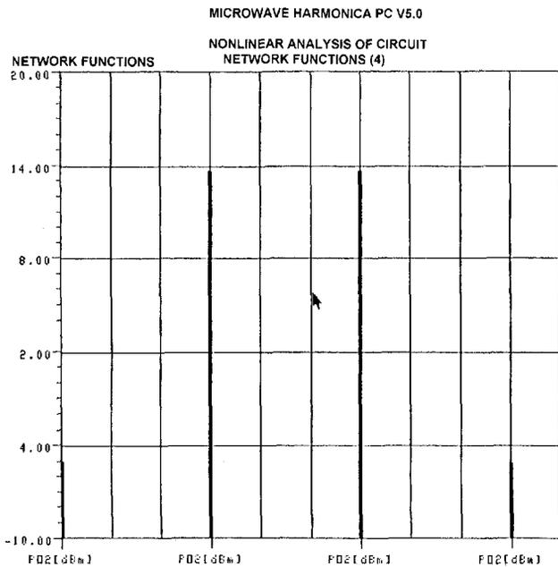
Figure 7. Simulated IM3, Pin = -16 dBm Two-Tone Avg.
