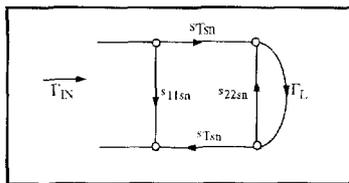
Figure 3. Flow-graph analysis used to determine the input reflection coefficient of the internal test fixture network.
