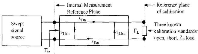
Figure 2. The one-port calibration process determines the errors represented by the various interconnecting system components. The error parameters are later used to correct mathematically any measured data.
