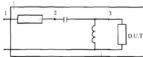
Figure 9. Three-element test fixture with D.U.T. connected between nodes 3 and 0. The input port of the fixture is between nodes 1 and 0.
