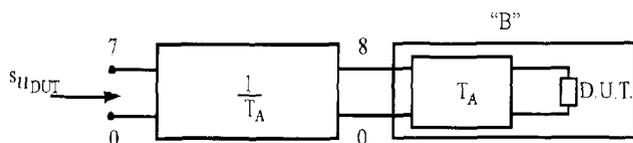
Figure 12. The measured one-port, including the test fixture parameters, is loaded into a one-port box "B" cascaded with the output port of a two-port containing the negated  $A$  ( $A^{-1}$ ).
