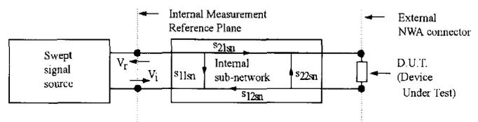
Figure 1. Simplified one-port network analyzer system block diagram. The imperfection of the internal sub-network introduces systematic errors to measurements.
