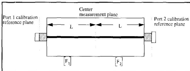
Figure 8. Two-port thru calibration fixture.
