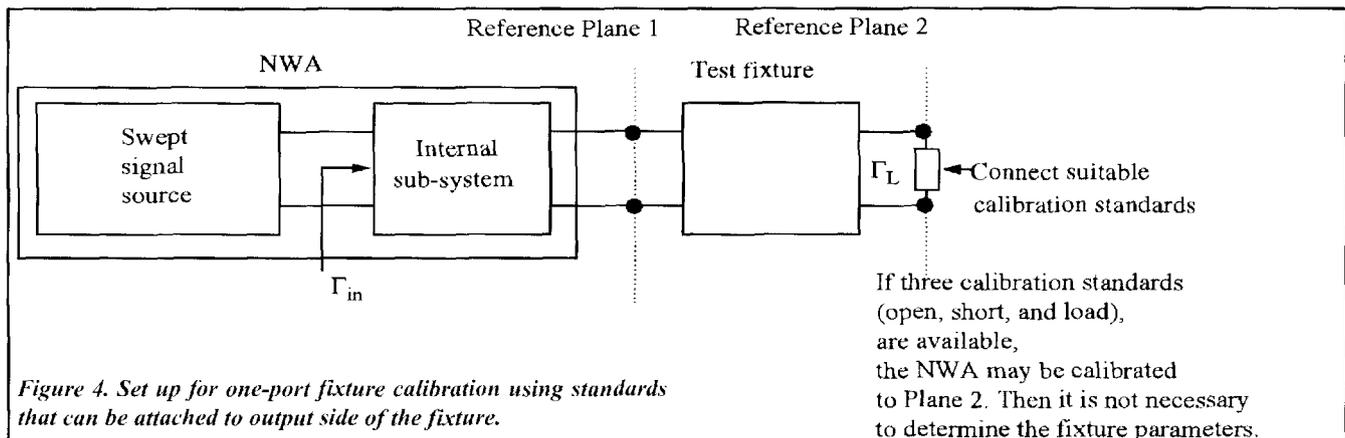
Figure 4. Set up for one-port fixture calibration using standards that can be attached to output side of the fixture.
