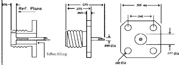
Figure A. Flange-mounted SMA connector (female) with Teflon dielectric ( $\epsilon_r = 2.14$ ).
