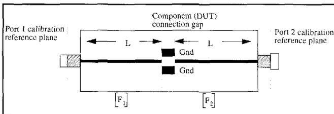
Figure 7. Two-port component measurement fixture.
