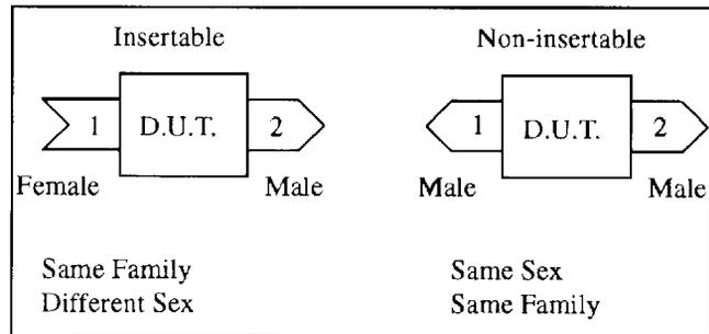
Figure 6. Classes of fixtures and devices under test (D.U.T.).
