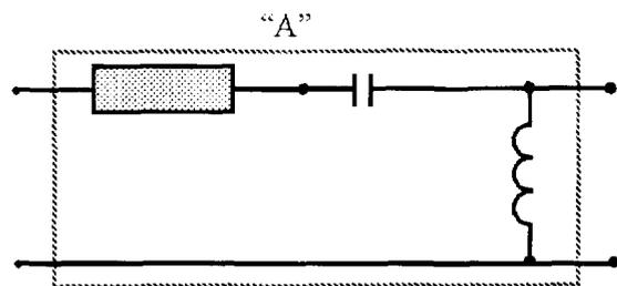
Figure 10. A section "A" which is negated in the calibration to compensate for the test fixture in which the D.U.T. is embedded.
