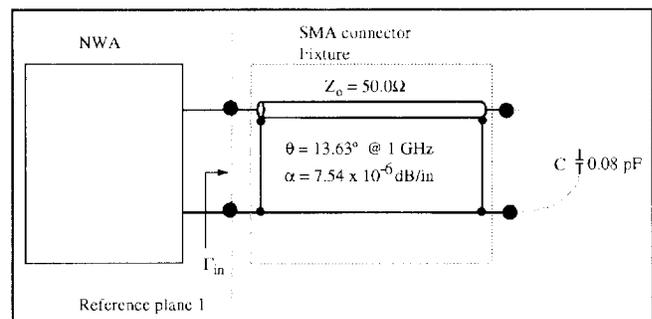
Figure 5. Fixture with optimized open SMA model values.
