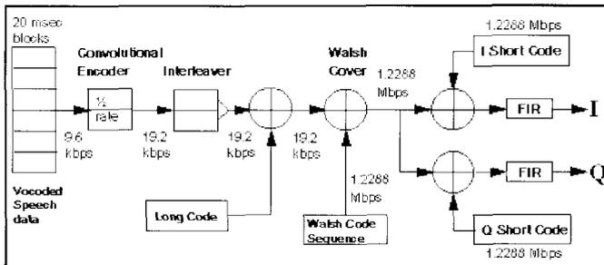
Figure 8. CDMA forward link physical layer.
