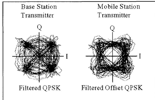
Figure 12. Constellation diagrams for CDMA modulation formats. (a) The base station transmitter uses filtered QPSK. (b) The mobile station transmitter uses filtered offset-QPSK.
