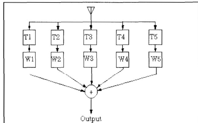
(b) RAKE receiver block diagram.
