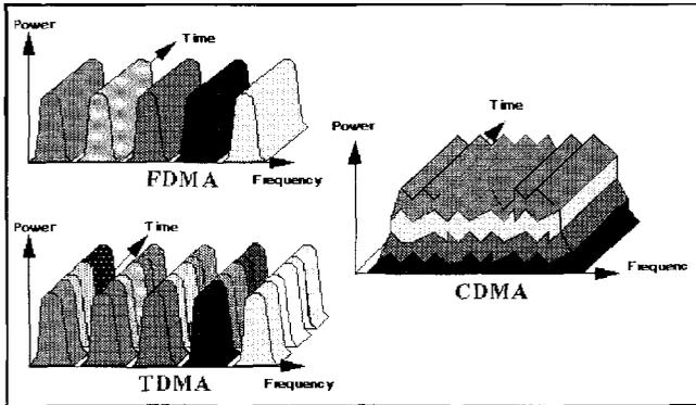
Figure 1. Cellular channelization methods. (a) Frequency Division Multiple Access (FDMA). (b) Time Division Multiple Access (TDMA). (c) Code Division Multiple Access (CDMA).
