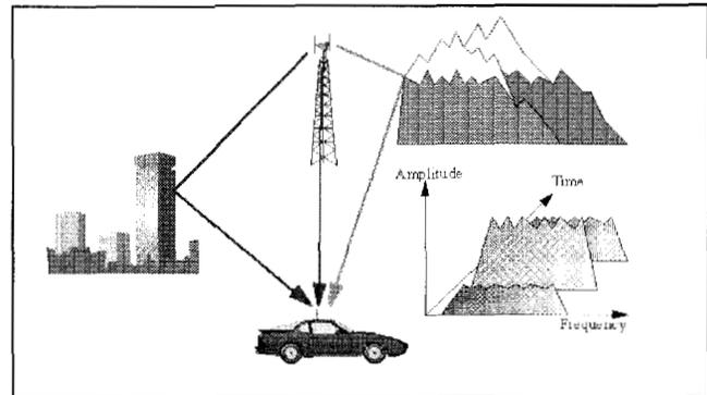
Figure 6. (a) The RAKE receiver takes advantage of multipath transmission to realize a form of time diversity.
