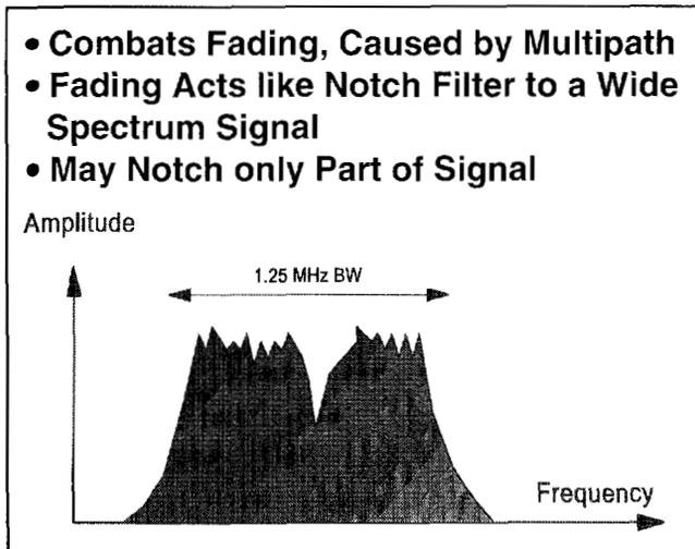
Figure 5. CDMA frequency diversity. The wide spectrum combats fading caused by multipath transmission. Fading has the effect of a notch filter to the wide-spectrum signal. Typically only a small part of the signal is lost.
