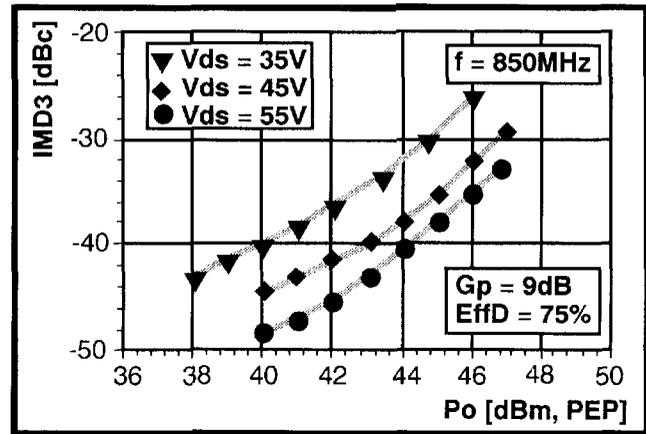
Figure 8. Class A Pulsed RF IMD3.
