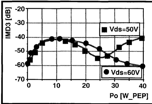
Figure 6. JFET IMD3 versus output power (watts PEP) at 215 MHz for 50 and 60 volt Vds.
