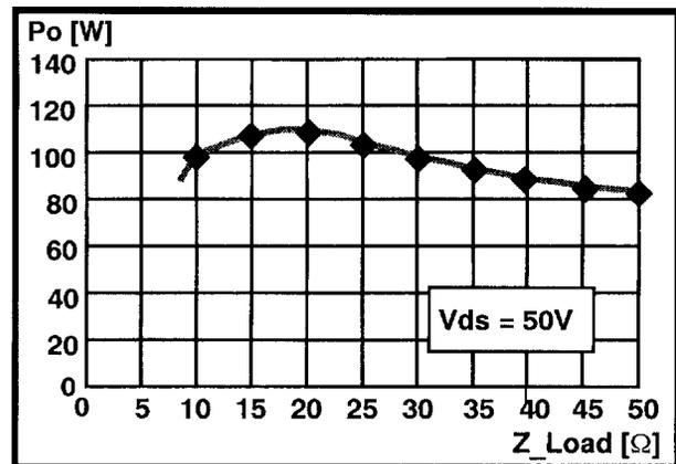
Figure 2. JFET output power as a function of load impedance.
