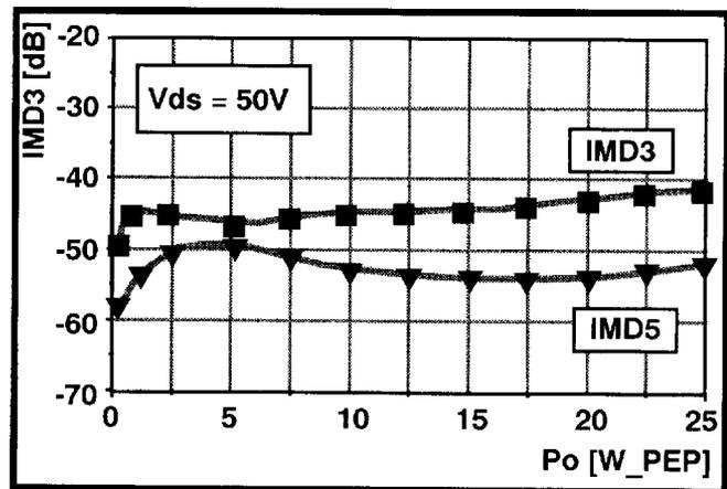
Figure 5. IMD3 and IMD5, f=30 MHz.
