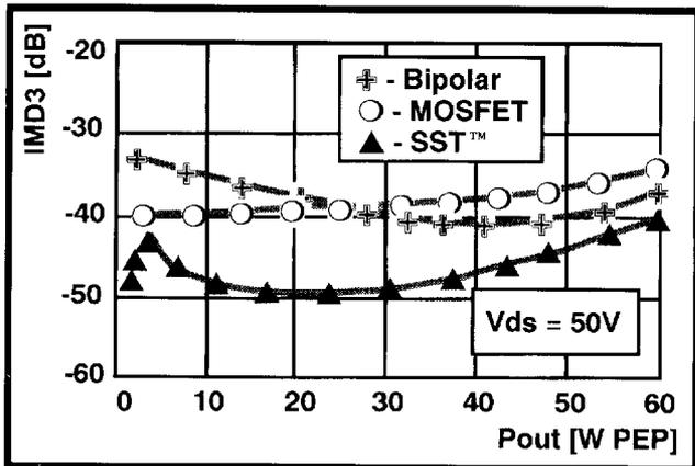
Figure 3. Class AB IMD3 Comparison.
