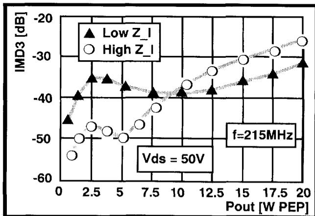
Figure 7. IMD3 versus load impedance.
