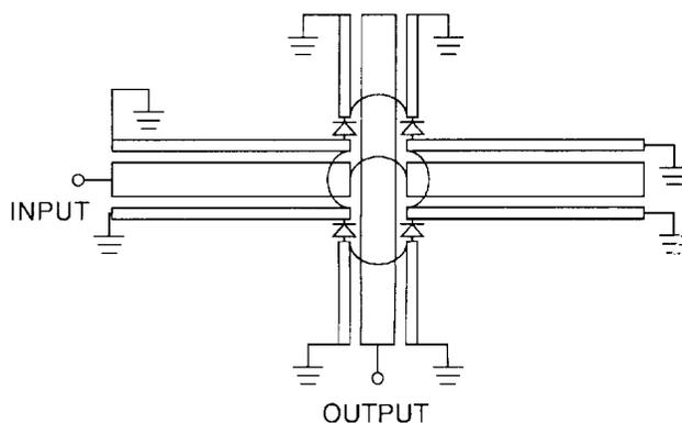
Figure 2. Diode frequency doubler in monolithic form.
