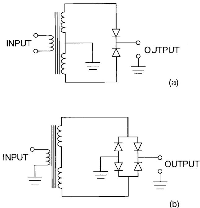
Figure 3. Two other possible bridge-rectifier multipliers: (a) a two-diode circuit and (b) a four-diode circuit using only one balun. A transformer cannot be used in circuit (b).
