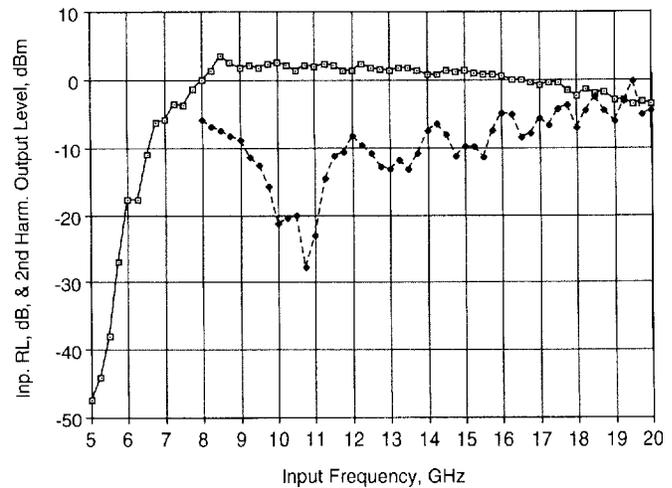
Figure 5. Second-harmonic output power (solid line) and input return loss (dashed line) of the diode doubler.  $P_{in} = 13$  dBm.
