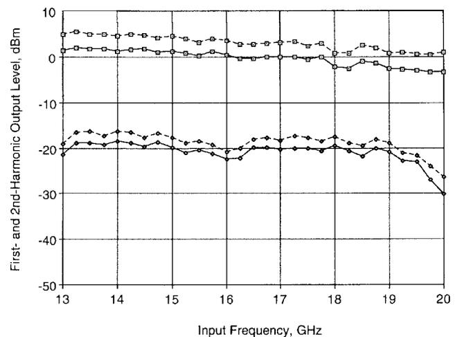
Figure 6. Fundamental-frequency and second-harmonic output power from 13 to 20 GHz at  $P_{in} = +16$  dBm (dashed lines).
