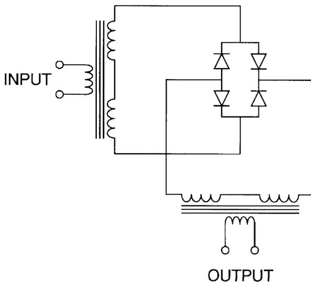
Figure 1. Diode multiplier in its ideal, transformer configuration.
