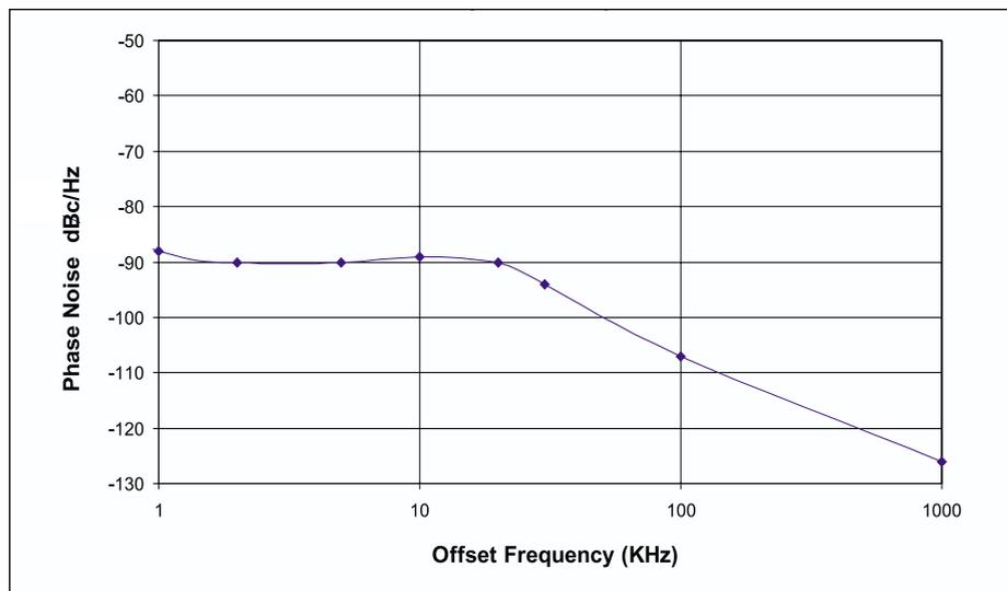
▲ **Figure 2. LMDS synthesizer noise data at 26.5 GHz.**
