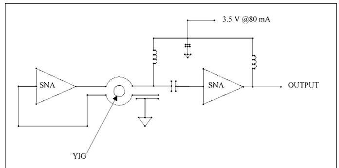
▲ Figure 3. IC-based oscillator circuit.
