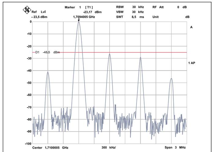
▲ **Figure 7. Carrier and sideband performance at low PCS band for the VMS-1710 model.**
