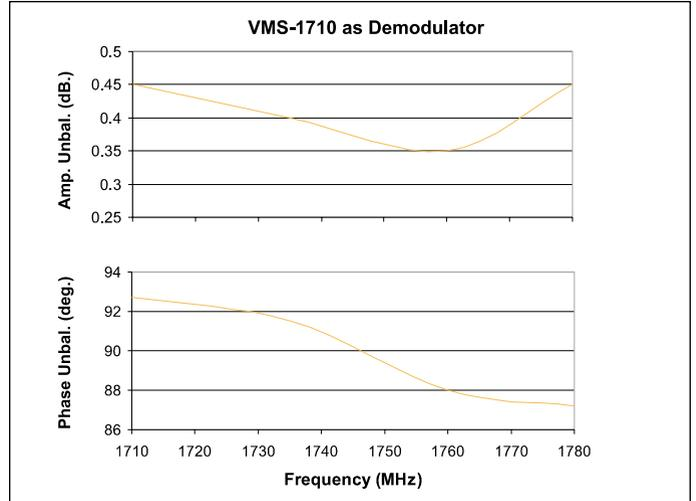
▲ **Figure 9. The amplitude and phase unbalances across the full band of 1710-1780 MHz.**
