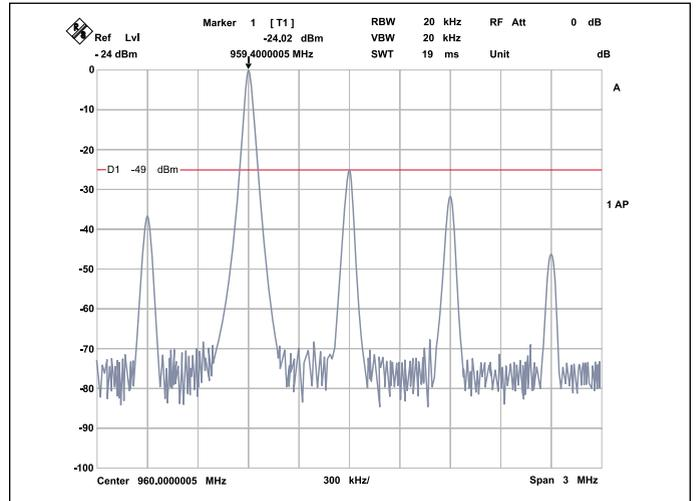
▲ **Figure 5. Carrier and sideband performance at high cellular band for the VMS-935 model**
