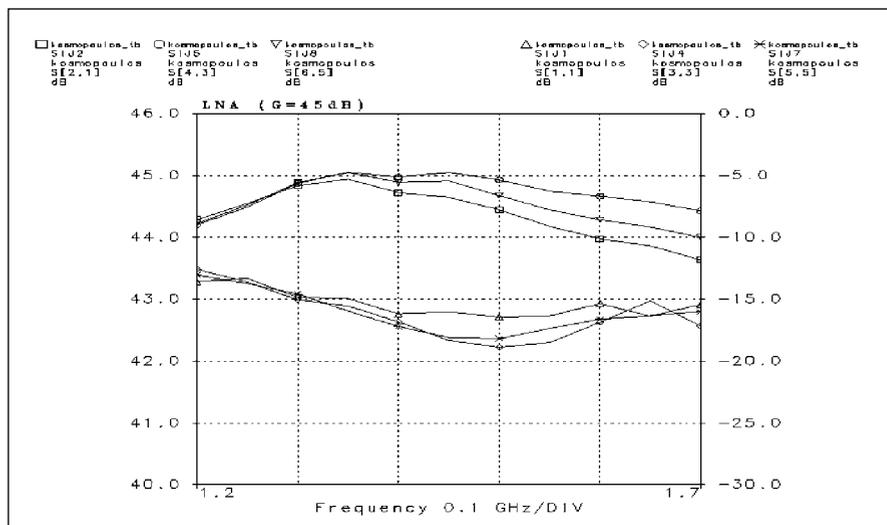
▲ Figure 8. S-parameters variation of LNA2 (triangle = -40° C; circle = +25° C; rectangle = +80° C).
