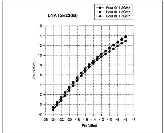
▲ Figure 3. Output power compression response of LNA 1 at 1 dB.
