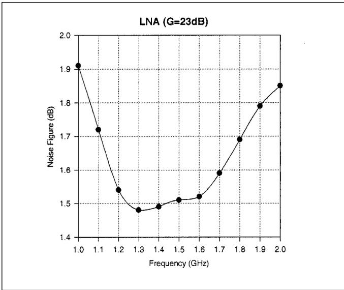
▲ Figure 2. Noise figure response of the first low noise amplifier design (LNA 1).
