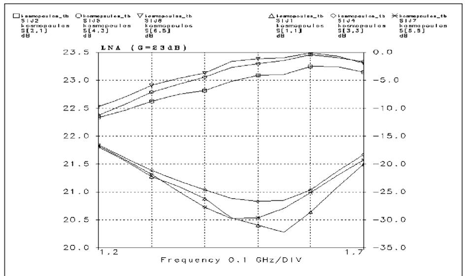
▲ Figure 7. S-parameters variation of LNA 1 (triangle = -40°C; circle = +25°C; rectangle = +80°C).
