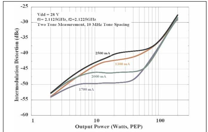
▲ Figure 6. MRF21180 IMD vs. power and  $I_{dq}$ .
