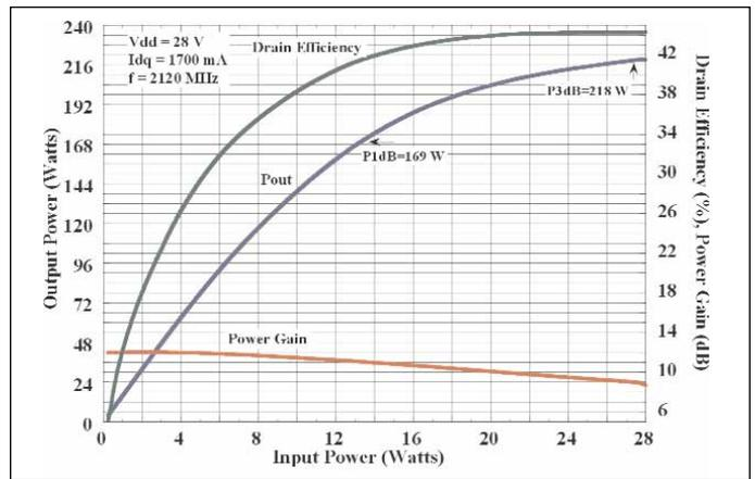
▲ Figure 2. MRF21125 output power vs. input power.
