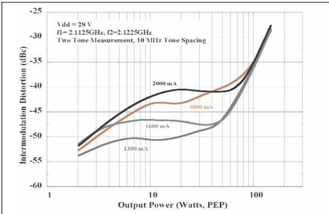
▲ Figure 5. MRF21125 IMD vs. power and  $I_{dq}$ .
