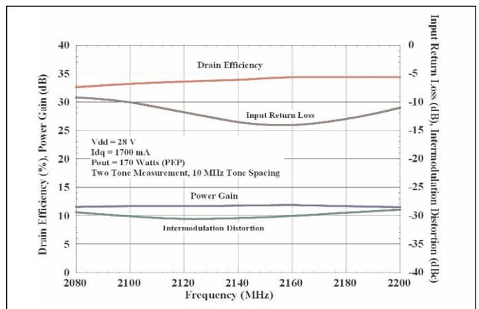
▲ Figure 4. MRF21180 two-tone performance vs. frequency.
