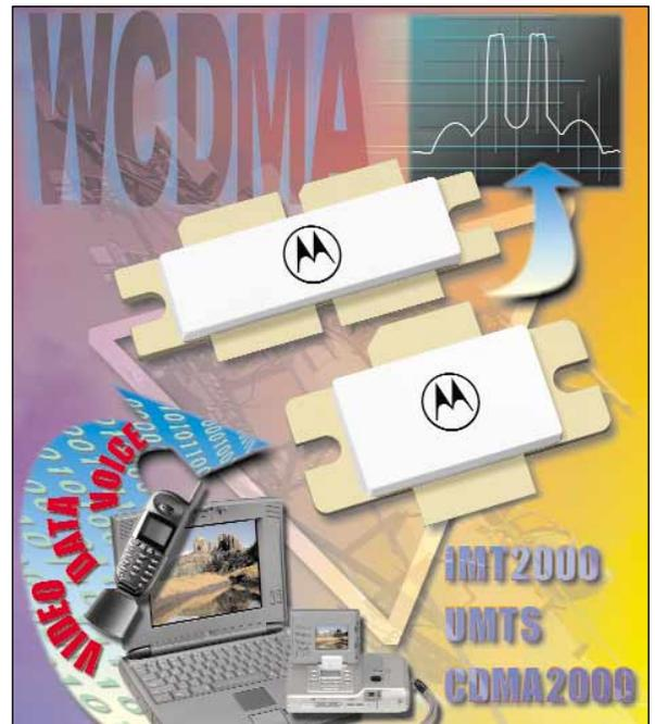
$IM_3$  of better than  $-30$  dBc is maintained across the band with an input return loss of better than  $-12$  dB and drain efficiency and power gain in excess of 33 percent and 11.5 dB respectively.
