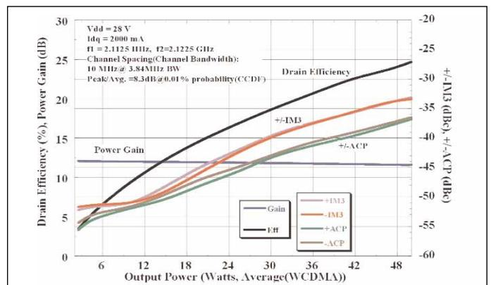
▲ Figure 8. MRF21180 ACP and  $IM_3$  performance vs. output power.
