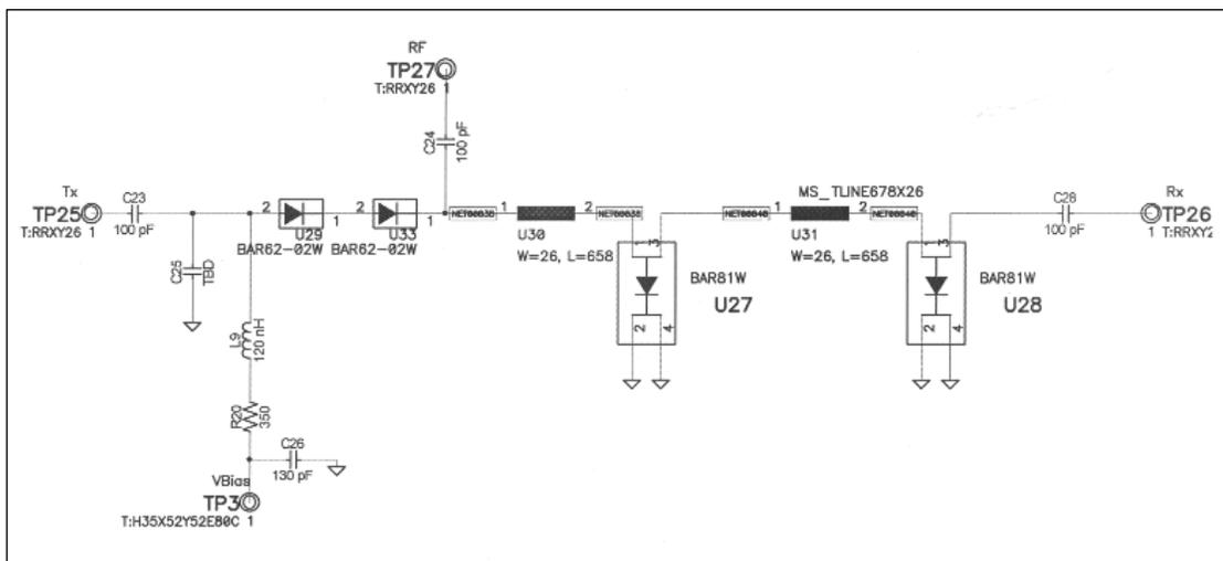
▲ **Figure 4. Schematic of a 2.45 GHz T/R switch with series diodes on the Tx port and shunt diodes on the Rx port.**
