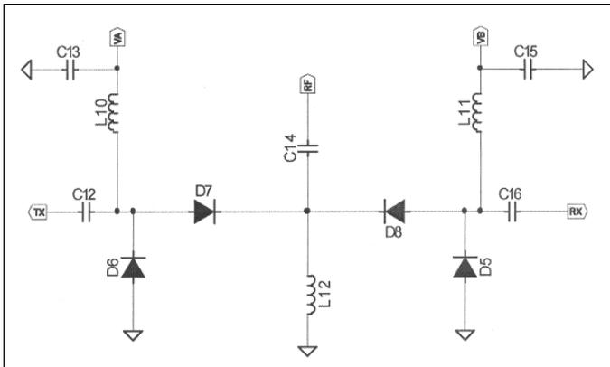
▲ **Figure 3. Series-shunt switch with high isolation.**
