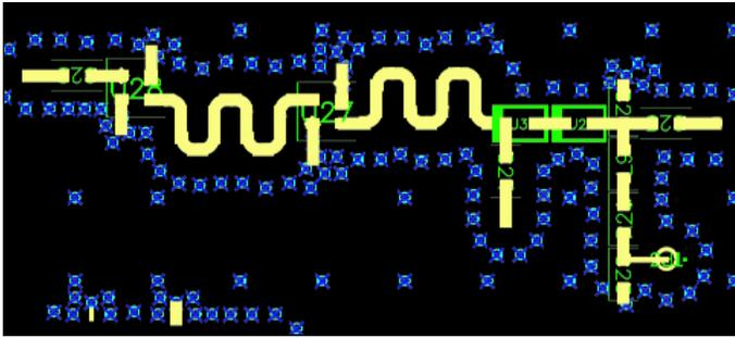
▲ Figure 5. Circuit board layout for the switch circuit shown in Figure 4.
