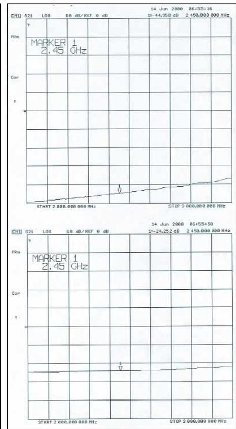
▲ Figure 12. Isolation between Tx and Rx ports.
