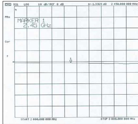
▲ Figure 9. Rx mode IL including cable loss.
