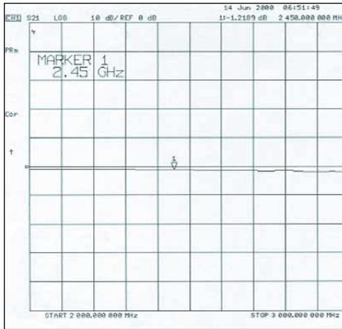
▲ Figure 8. Tx mode IL including cable loss.
