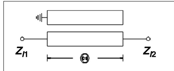
▲ **Figure 1. A directional coupler with coupled and isolated ports terminated in short and open.**
