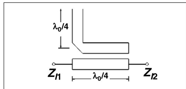
▲ **Figure 2. Short at the isolated port is accurately realized with open quarter wave stub**
