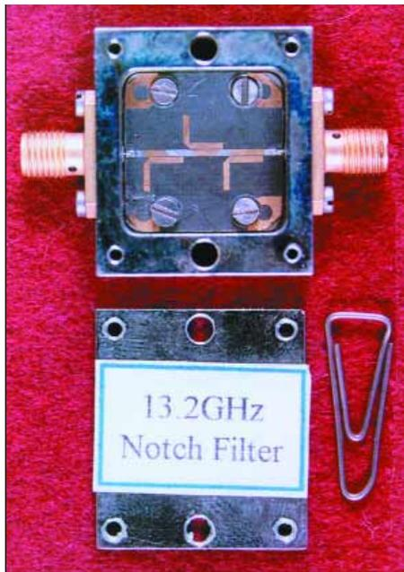
▲ Figure 7. A simple microstrip notch filter.
