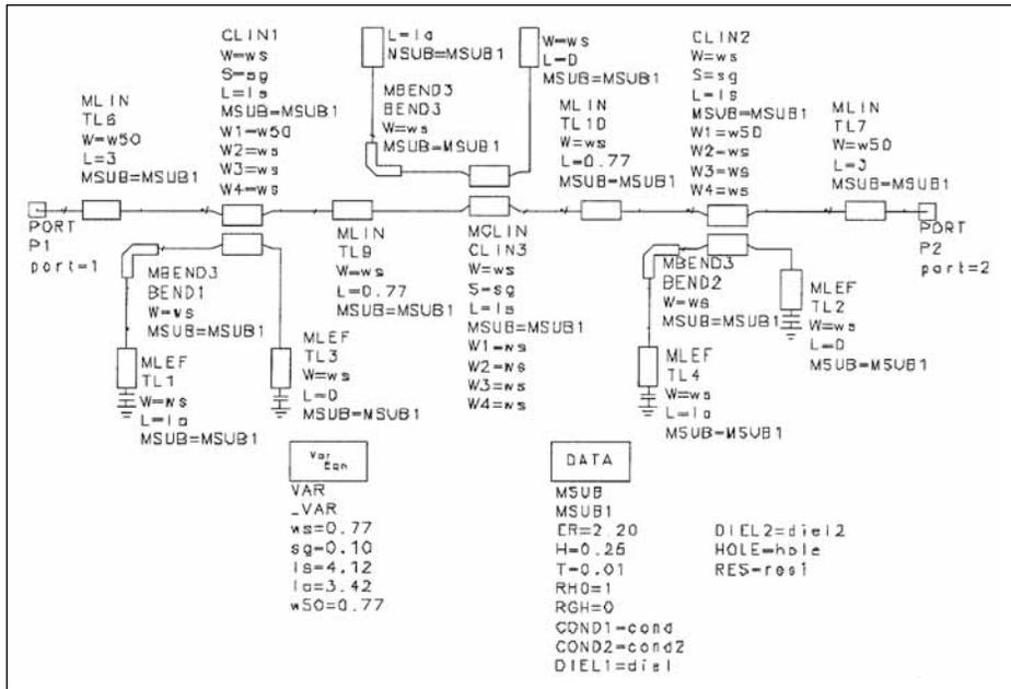
▲ Figure 3. *Libra* schematic of the notch filter.
