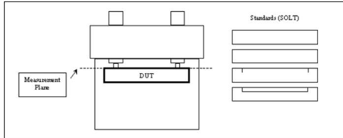
▲ Figure 1(a). A bandpass filter test fixture.
