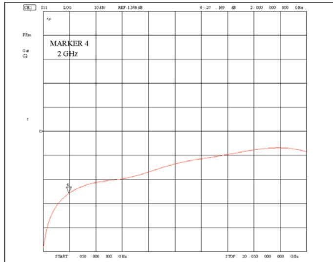
▲ **Figure 2(b).** Frequency response of the fixture viewed in the time domain with gating on.
