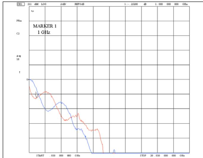
▲ **Figure 6. Two-way insertion loss of the through standard.**
