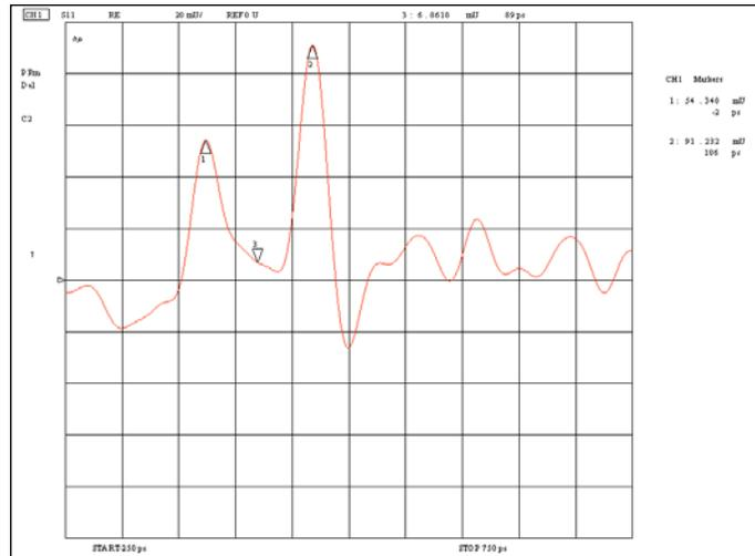
▲ **Figure 5. Offset impedance, identified with markers between the two pogo-conductor transitions.**
