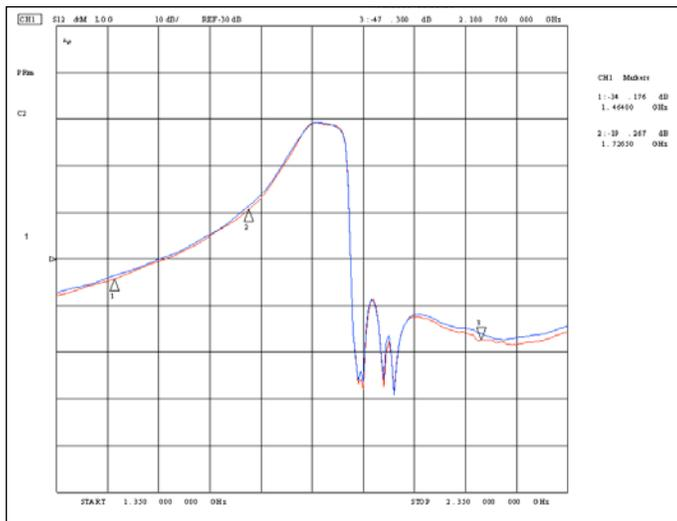
▲ **Figure 8(a).** The initial calibration kit definitions produced the responses in (a).
