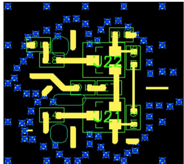
▲ **Figure 2. Layout of the PIN diode based VCA.**
