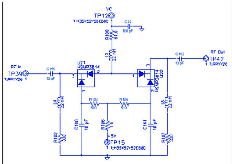
▲ **Figure 1. Schematic of the PIN diode-based VCA.**
